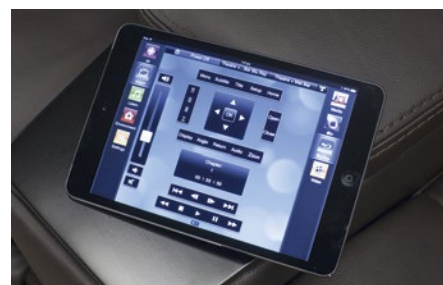
The iPad control for this home theatre uses the Savant control system with special buttons for 'Movie Start', 'Popcorn Time' and 'Movie Finish'. The main equipment is kept out of sight (below) in a high-quality rack with ease of service access.
