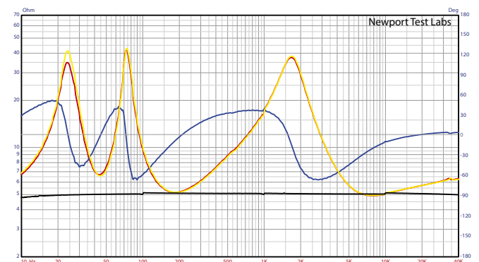
Graph 4. Impedance modulus of left (red trace) and right (yellow trace) speakers plus phase (blue trace). Black trace under is reference 5-ohm precision calibration resistor.
