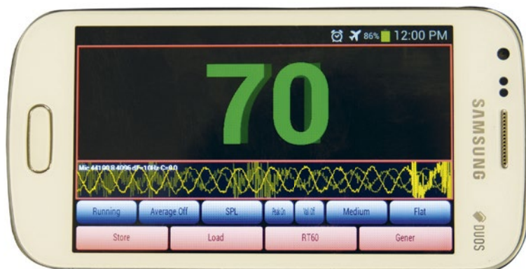
Photo 1: This illustration shows the Android version of the Audio Tool RTA app [ http://tinyurl.com/audiotool-app ] running in its SPL mode on a Samsung GT-S7562 Smartphone, measuring a 100Hz warble tone (from Stereophile Test CD2, Track 16, Index 4) at 70dB SPL. (The end result of Step 3 of the calibration process.) You can see from the blue 'soft' keys that the averaging is set to 'Off', the mode is 'SPL', Meter Response is set to 'Medium' and that weighting is set to 'Flat'. The two small tabs visible between the tabs that show 'SPL' and 'Medium' are for Peak Hold (On/Off) and Valley (On/Off). For this measurement, either button can be in either mode, as they don't affect the measurement.
