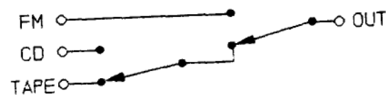
FIGURE 8-24: Switching three sources with two switches.
