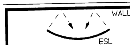
FIGURE 14-13: Poor position—Rear wave reflects through dipole.
