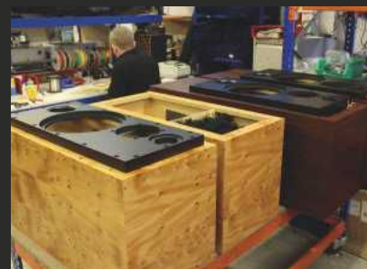
These hand-made drive units are about to be fitted into the cabinets in ATC's Cotswolds-based factory
