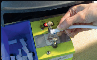
5 The cable's outer sleeve is heat-cut using this special machine, ready for fitting
