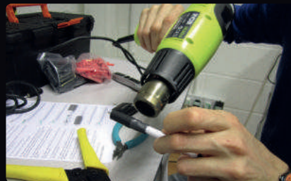
6 The sleeve is pulled up to the end of the plug, and heat shrink is fitted using a special heat gun
