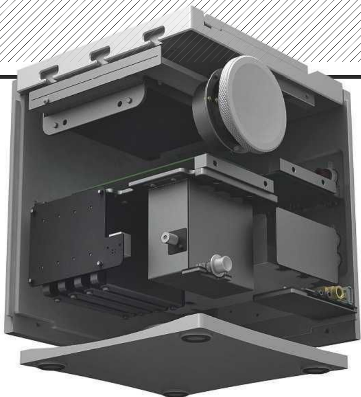
LEFT: Internal view reveals quite a lot of fresh air between the CD drive and rest of the player electronics. Lower down is the dock for up to four SSD hard drives [left], and the battery power supply [right]
