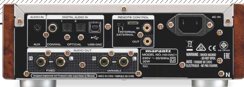
ABOVE: As well as the USB Type-B for asynchronous connection to a computer, the Marantz has both optical and coaxial S/PDIF digital inputs plus an analogue in via a miniature jack. Separate fixed and variable RCA outputs are provided
