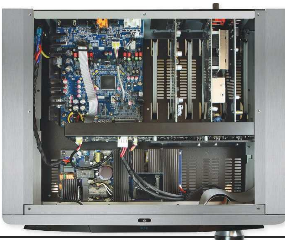
RIGHT: NAD's modular architecture sees optional HDMI, Bluetooth, Ethernet and Wi-Fi input cards loaded into its expansion bays (top right). Analogue inputs are processed digitally
