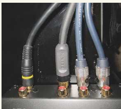
ABOVE: Rear of the switch box showing three input cables and black output lead
