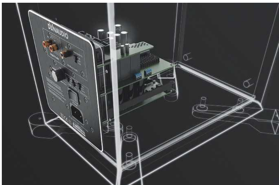
ABOVE: Hidden behind the control panel are the active electronics. From the input, signals go to the DSP that provides the crossover and in turn feeds three 150W Class D amplifiers
