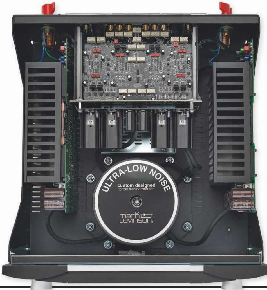
RIGHT: A single 900VA transformer (with dual secondaries) feeds independently-regulated supplies for the 12-transistor strong Class A/B power amp(s) and DAC section
