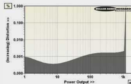
ABOVE: Continuous power output versus distortion up to 1% THD into 25ohm 'headphone' load
