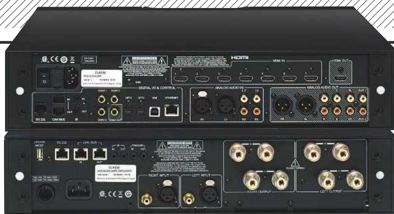
ABOVE: With balanced [XLR] and unbalanced connections on both units, the SSP has a plethora of inputs, including HDMI, coaxial and optical digital, USB and analogue. Numerous HDMI sockets and analogue outputs provide for multichannel operation
