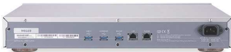
ABOVE: Rear panel plays it simple: network and direct player Ethernet connections, plus USB ports dedicated to expansion, back-up, loading of content and replay via an external DAC (this is a USB 3.0 compatible port)
