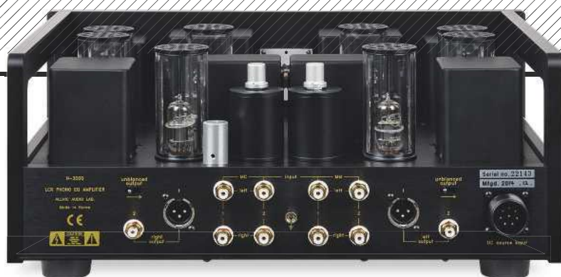
ABOVE: Four cartridge inputs are offered, on unbalanced RCA phono sockets, while unbalanced and balanced (XLR) outputs are offered, selected by two small switches. The chunky multi-way input on the right accommodates the PSU's umbilical cable
