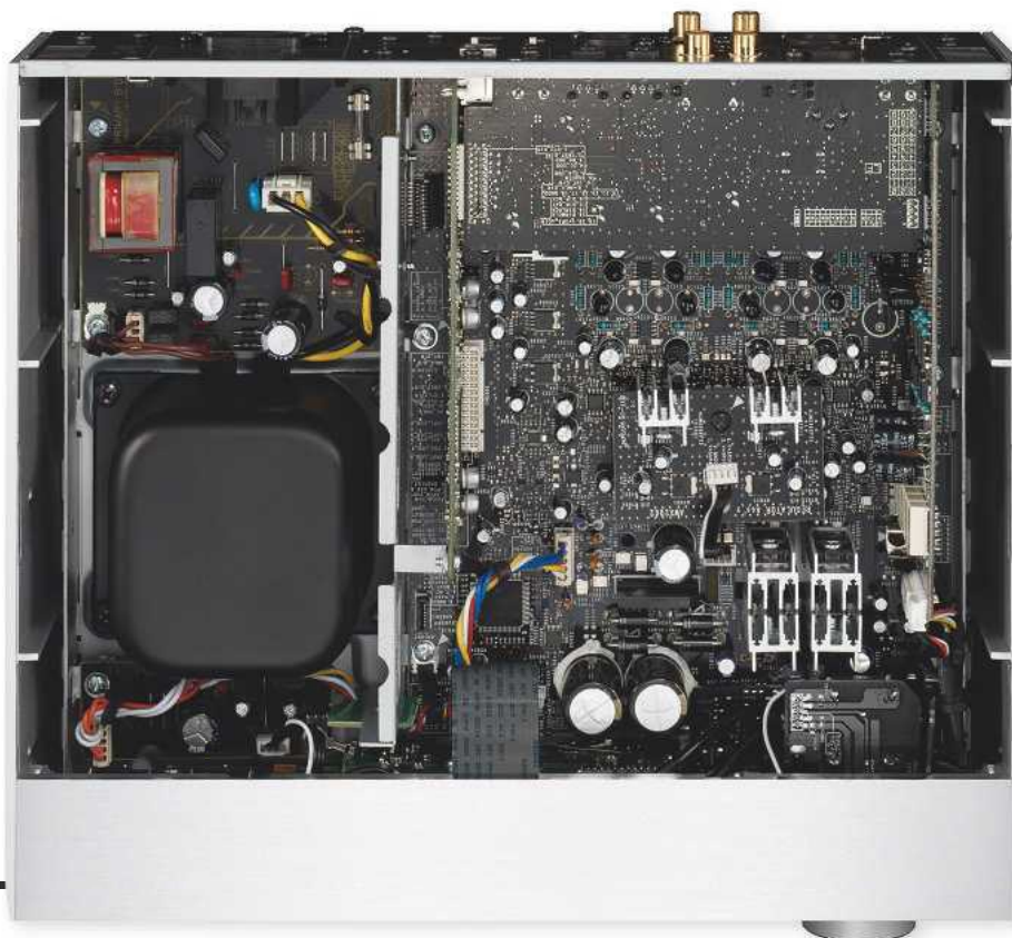
RIGHT: The U-05's packed interior includes a hefty linear PSU, a pair of (8-channel) ESS Sabre ES9016S '32-bit' DACs and fully balanced analogue stages for line and headphone outs
