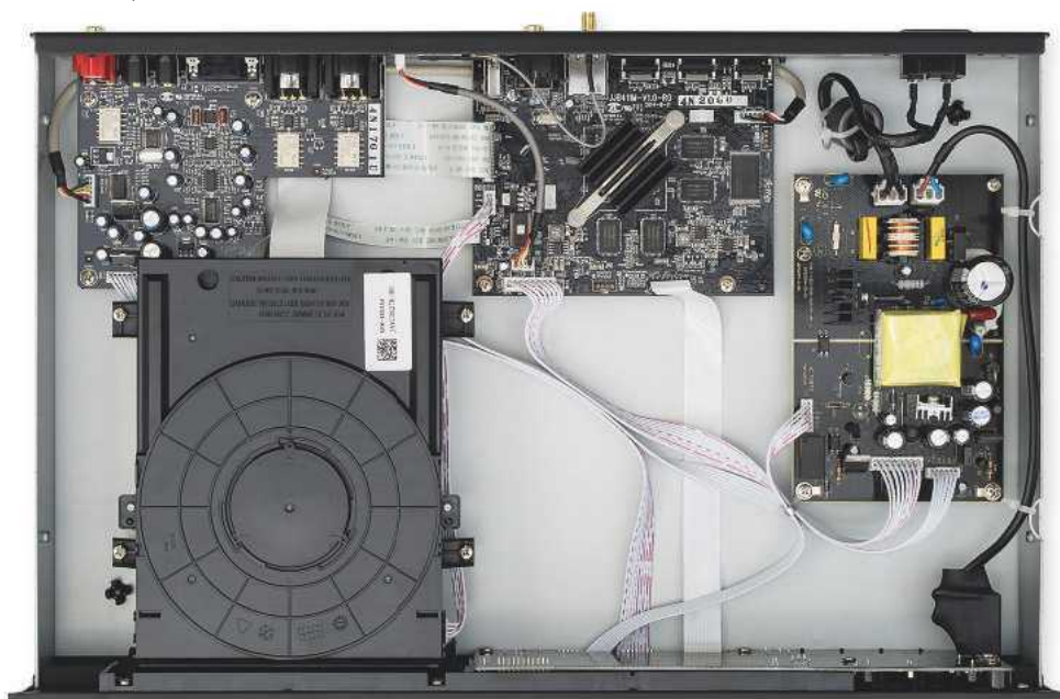
RIGHT: Three PCBs (from right to left) include a switch mode PSU; embedded PC/DSP board handling all network/USB processes; and audio board with Burr-Brown PCM1794 DAC
