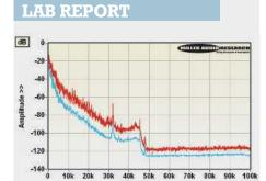
This looks like a 96kHz recording but there remains a lot of spurious noise and ultrasonic 'clutter' in addition to peaks at 20kHz, 32kHz and 46kHz. How much of the post-20kHz content is 'real' and how much is distortion from limiters, etc? PM
