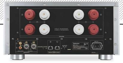
ABOVE: SE-R1 has twin sets of hefty loudspeaker terminals, with front-panel selector: as well as the Digital Link connection there are analogue inputs on RCA and XLR
