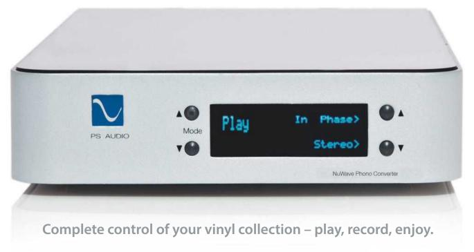
The NPC combines a state-of-the-art pure analogue phono pre-amplifier with a high-end analogue PCM/DSD converter. Play anything from your turntable or analogue source via the NPC into your pre-amp. Or record your vinyl collection through the NPC onto your computer and play it back via a DAC.
