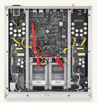
ABOVE: Inside the Melco N1Z media player - two 'Audio Grade' solid-state drives flanked by separate switched-mode PSUs
