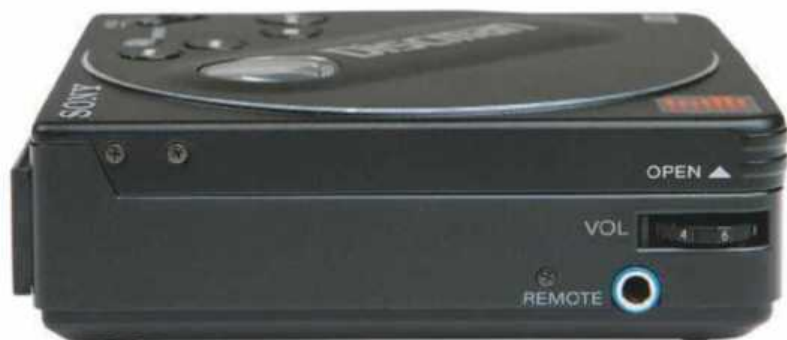
ABOVE: The volume control was positioned so that it could still be reached with a 12cm CD loaded while the blue 3.5mm jack socket accepted a wired remote control
