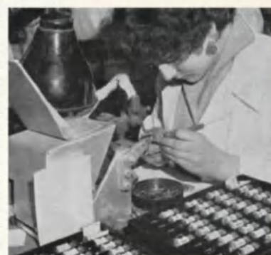
ABOVE RIGHT: Fig 5 – this machine transfers mica and filament to an air-hammer and then, with a puff of compressed air, to storage boxes
