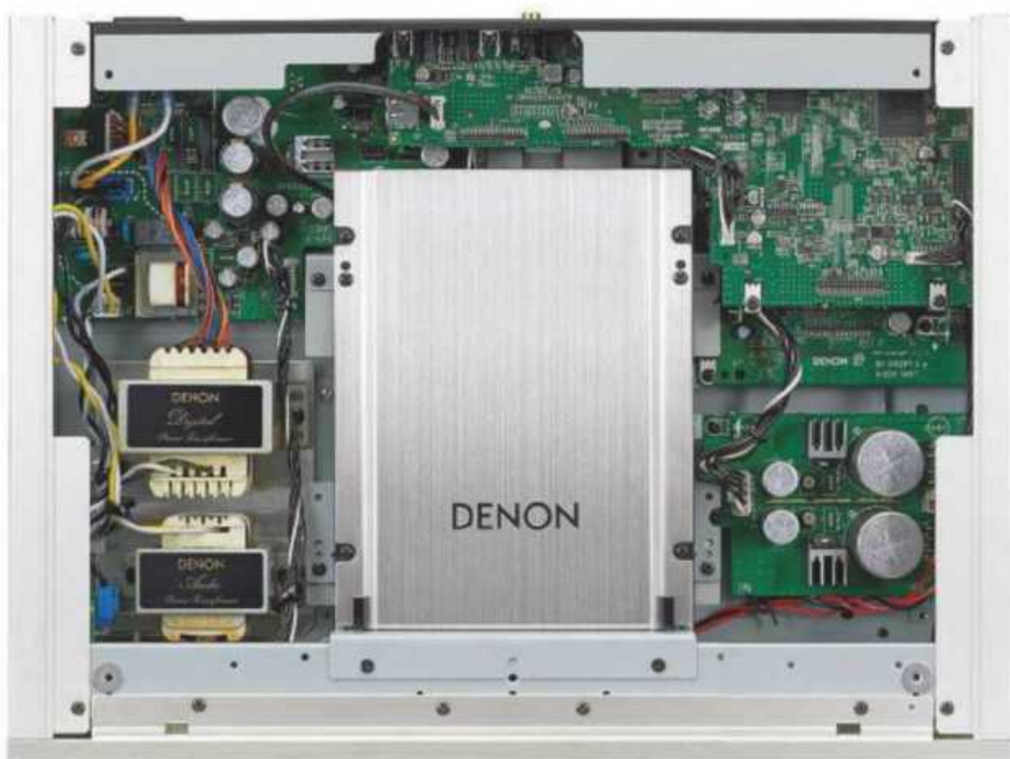
RIGHT: Separate power supplies feed the DVD transport mechanism, digital processing and analogue stages. Burr-Brown's proven 192kHz/32-bit DAC handles LPCM and DSD data
