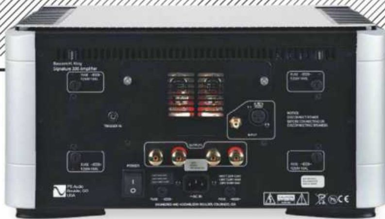
ABOVE: A single balanced XLR input is joined by parallel sets of 4mm compression-fit speaker connections. Note 12V trigger comms and removable triode tube 'hatch'
