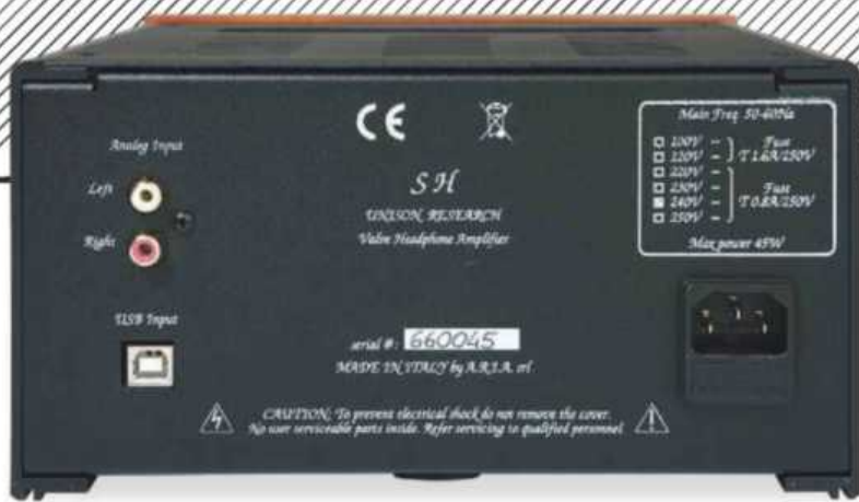
ABOVE: No balanced analogue inputs (or outputs) but simply one set of single-ended RCAs with a USB Type-B port for delivery of music files via a computer or media server
