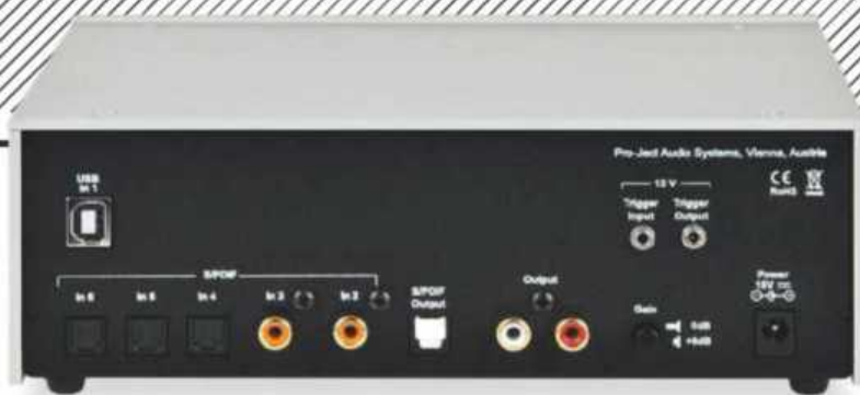
ABOVE: Unbalanced analogue outs on RCAs offer two gain settings and are joined by DSD-ready USB, three optical and two coaxial S/PDIF digital inputs. Trigger connections are included while 18V power is supplied via a wall-wart supply
