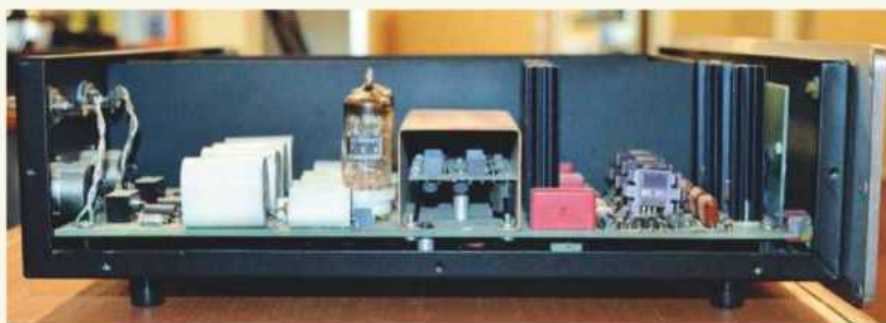
ABOVE: Side view of the Sonic Frontiers SFD-2 showing the analogue output stage with tubes
