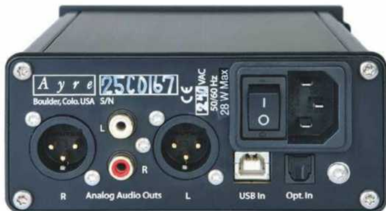
ABOVE: S/PDIF optical input plays second-fiddle to the 384kHz/DSD128-compatible USB input. Fixed and variable analogue outputs offered on RCAs and balanced XLRs
