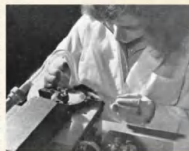
LEFT: Fig 2 – here precision machines are used for winding the very fine grids needed for miniature and sub-miniature valves. These are then cut into sections
