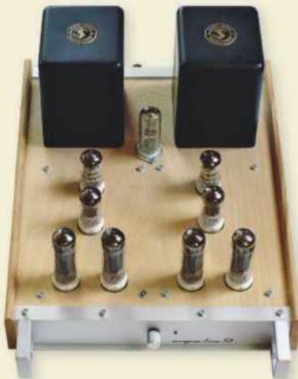
ABOVE: Stereo Mullard 5-10 amplifier built using the Mullard circuit from 1954
