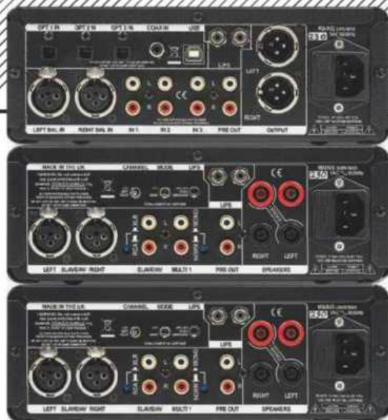
LEFT: Balanced XLR outs on the pre (top) are matched by XLR ins on the power amp(s), the former also offering XLR and three RCA ins, USB and S/PDIF digital ins (three optical, one coax). BFA 'short-proof' speaker outlets and LIPS connections complete the package
