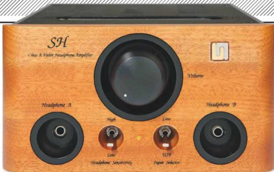
LEFT: Controls are minimal: between the twin output sockets and to either side of the central volume control are toggle switches to adjust gain and select digital or analogue input
