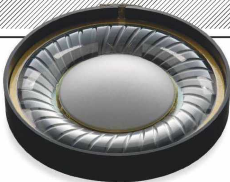
ABOVE: Pioneer's 50mm drive unit combines a 25 \mu m-thick aluminium dome with a PEEK surround. 'Parker Ceramic Coating' is applied to enhance the dome's stiffness
