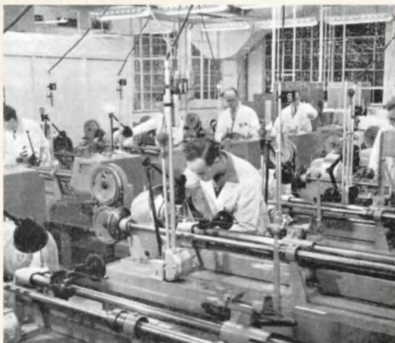
LEFT: Fig 2 – here precision machines are used for winding the very fine grids needed for miniature and sub-miniature valves. These are then cut into sections
