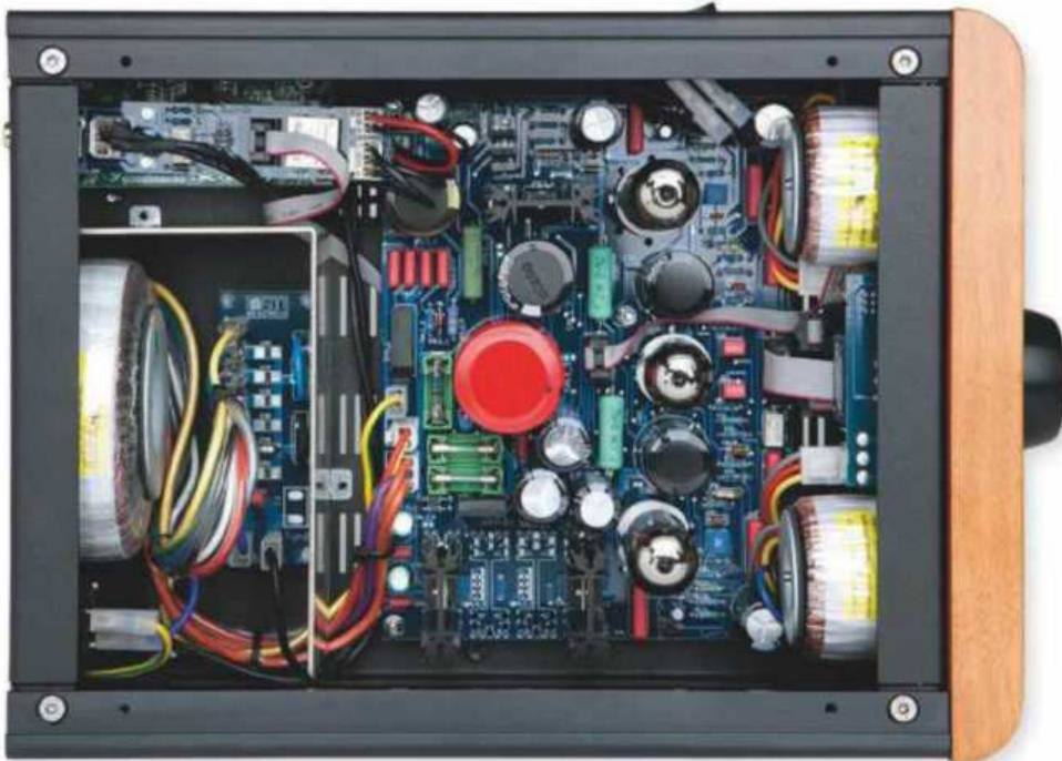
RIGHT: The EL84 output tubes, configured in triode mode, drive a pair of headphone sockets via toroidal coupling transformers – visible here far right. The PSU transformer is on the far left
