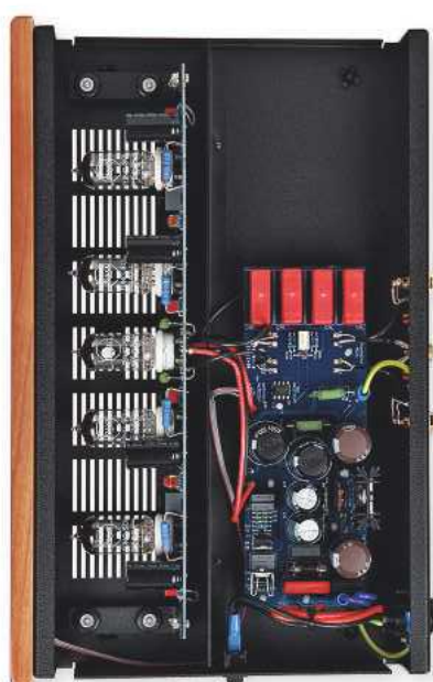
ABOVE: Five ECC83 double-triodes are shared between input buffering and line output stages. RIAA eq is passive
