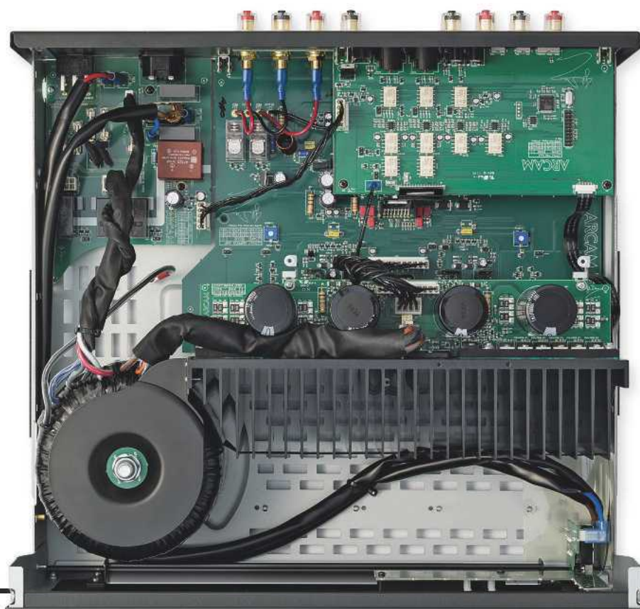
RIGHT: A single 1.5kVA toroidal power transformer has multiple secondary windings. These feed the lower and higher supply rails that service Arcam's Class G output stage
