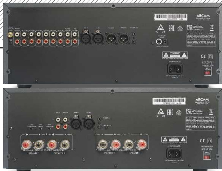
ABOVE: A lot of blank metal on the rear of both preamp and power amp indicates the simplicity here. Worth noting (and using) are the balanced inputs and outputs for the best sound, while the C49 has a power output for Arcam's r-Series add-on DACs
