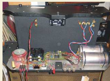
ABOVE: Reassembled unit showing amp (left) and speaker inverted to show underside of amp
