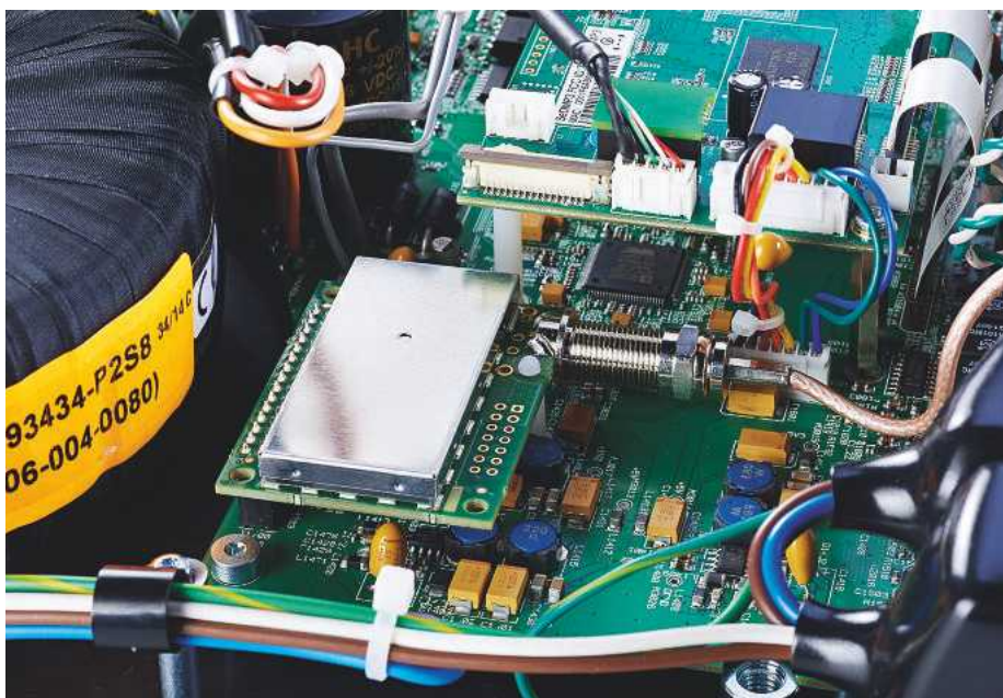
ABOVE: Naim's UPNP network connection is screened on its own daughter board and will accept 32-bit floating-point WAV files as well as standard-resolution 2.8MHz DSD files (also via USB-A input)
