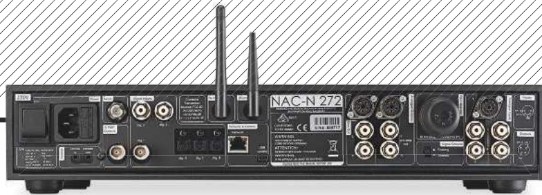
ABOVE: Phono (RCA) connections and DIN sockets are included for analogue input and output, but Naim also offers six digital inputs (three coax/three optical), a wired Ethernet connection and three antenna inputs: Wi-Fi, Bluetooth and optional radio
