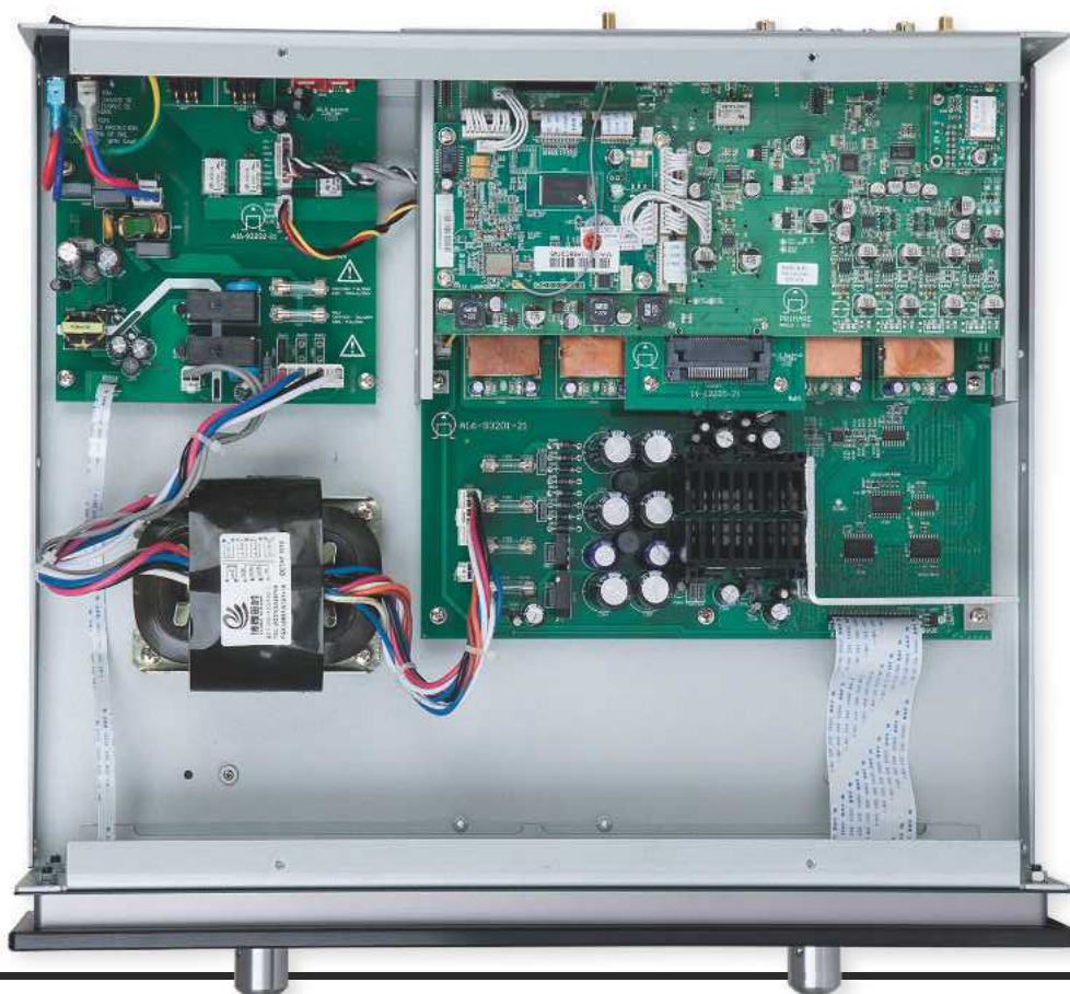
RIGHT: PRE32 preamp including additional MM30 DAC/streamer media board and Bluetooth receiver, installed via a slot on the amp's rear panel to sit above the main PCB
