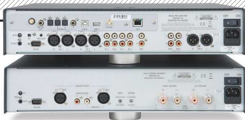
ABOVE: PRE32 ticks lots of analogue and digital boxes with four S/PDIF, two USB, Ethernet, Wi-Fi and Bluetooth inputs plus balanced and unbalanced analogue in/outs. The A34.2 power amp offers XLR and RCA inputs (note bridged mode toggle switch)
