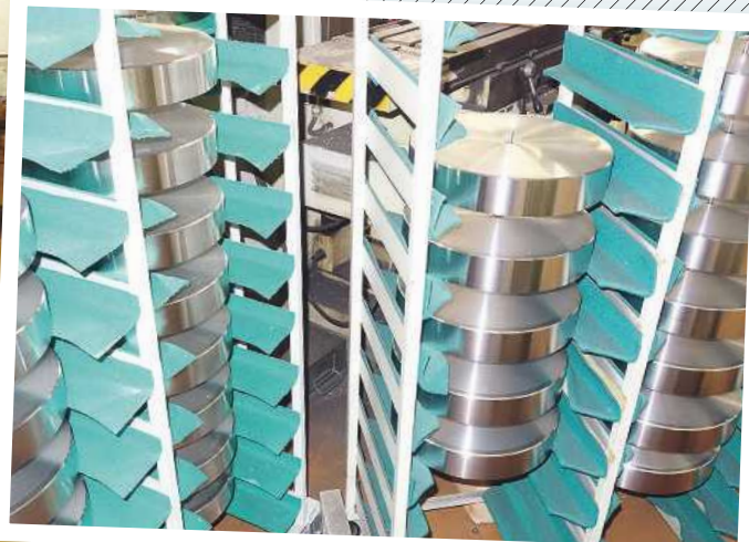
ABOVE: Stacks of all-metal platters fresh from finishing and awaiting balancing and matching to the turntables
