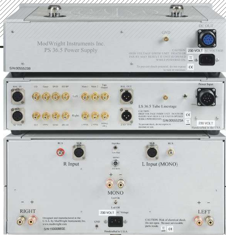
ABOVE: Rear view shows the preamp's balanced inputs and outputs [centre box], while the unlabelled toggle switch is a ground lift. On the power amp [bottom], the small toggle switch is for high/low bias, the larger one for bridged mono operation
