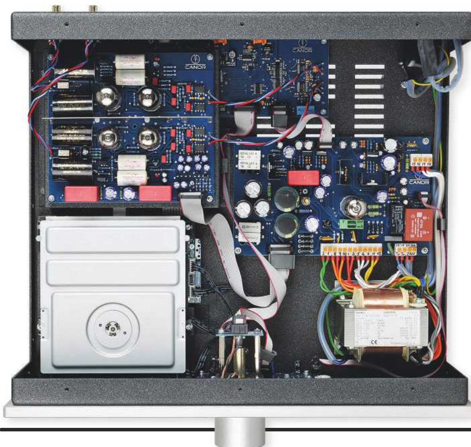
RIGHT: A popular and proven StreamUnlimited CD mech feeds two Burr-Brown PCM1792 DACs that drive the tube analogue output stage. Note the valve-rectified (EZ81) power supply
