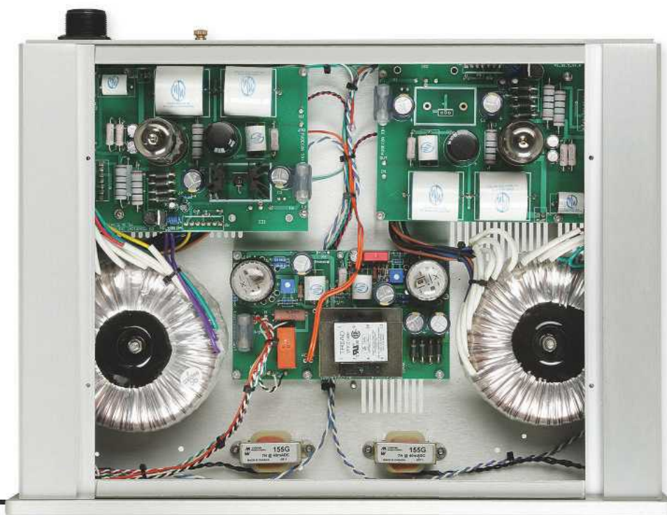
RIGHT: Inside the PS 36.5 power supply unit, which provides 'dual mono' power for the LS 36.5 preamp. Next to each of the rectifier tubes is a smaller voltage regulator tube
