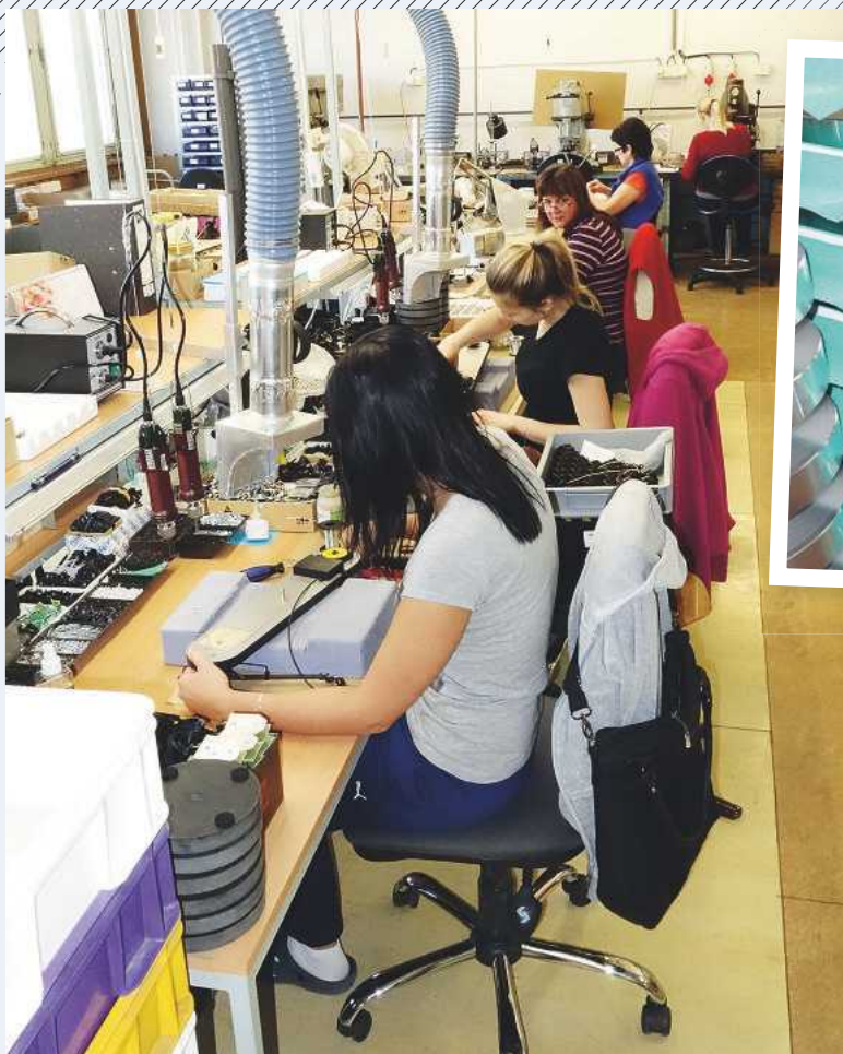
ABOVE: Stacks of all-metal platters fresh from finishing and awaiting balancing and matching to the turntables
