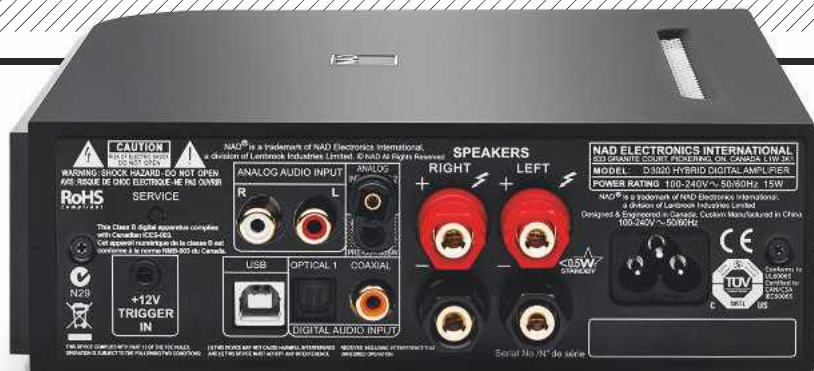
ABOVE: Comprehensive digital input options include a MacBook optical jack; there are two analogue inputs – the second sharing the 3.5mm MacBook jack socket
