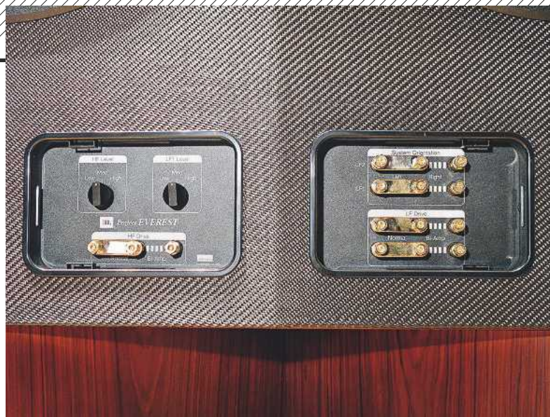
ABOVE: Cover plate on the baffle conceals switches for tweaking HF/LF levels, and links to handle the speaker and disable the network for active drive
