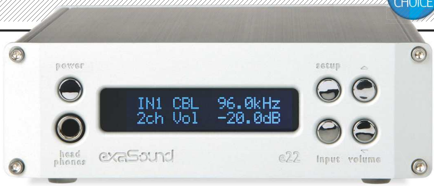
ABOVE: Front panel has a headphone socket and buttons for accessing the setup menu, input selection and volume up/down. Display indicates incoming data type and sampling rate
