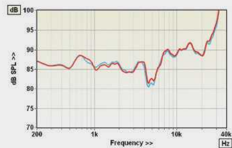
ABOVE: Forward response shows a declining output to the 4kHz crossover with a strong treble thereafter
