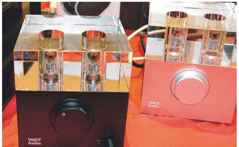
Woo Audio's WA7 'Fireflies' headphone amp drew plenty of enthusiastic attention in a big ground-floor hallway exhibit. The Class A valve beauty includes a built-in 32-bit/192kHz USB DAC and costs $999 with a solid-state power supply or $1399 with the WA7tp vacuum tube supply, which is shown to the right of the picture. www.wooaudio.com
