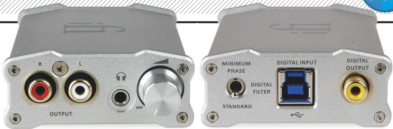
ABOVE: Front panel has just line and headphone outputs and volume/power control, while at the rear the filter switch and coaxial digital input straddle the USB-B connection
