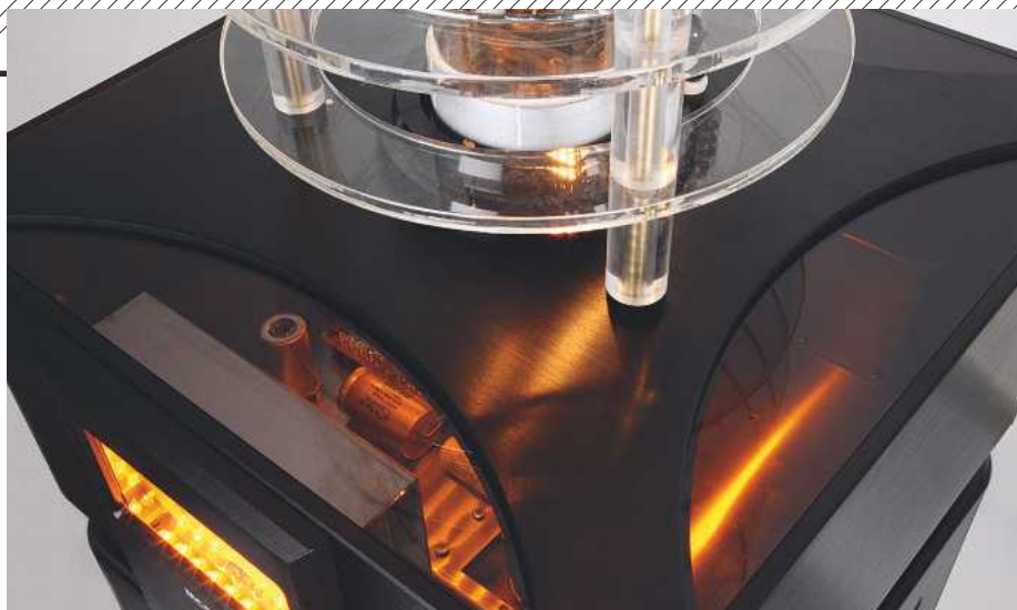
ABOVE: Ming Da's hard-wired input and driver stages are visible inside an illuminated bay – Jensen electrolytics and Jinvina resistors partnering an ECC83 double-triode and Tung-Sol 6L6 tetrode
