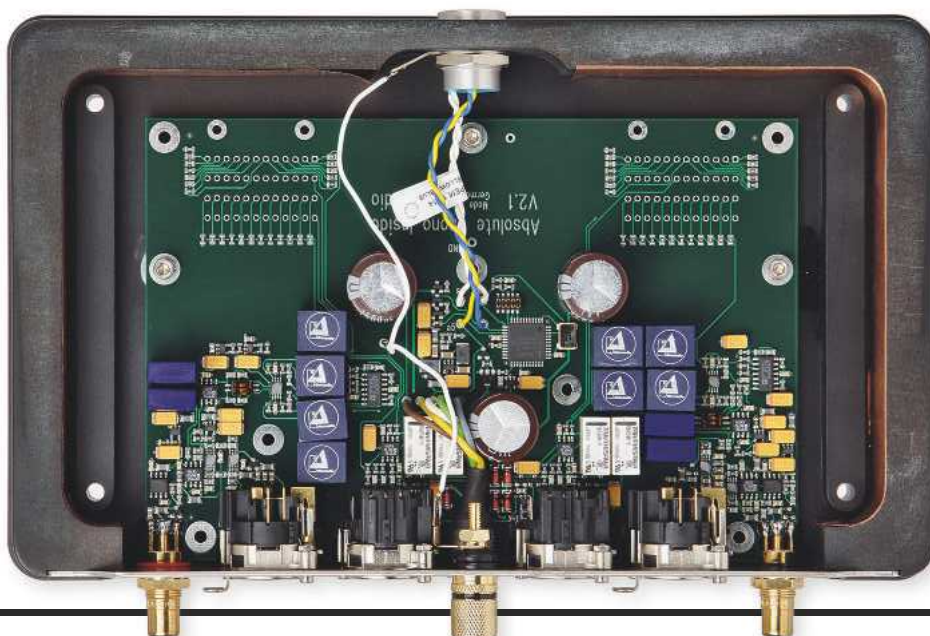
RIGHT: Dual-mono and fully balanced, Clearaudio's current amplification is based around OP275/OP484 op-amps with quality passives for the RIAA equalisation stage
