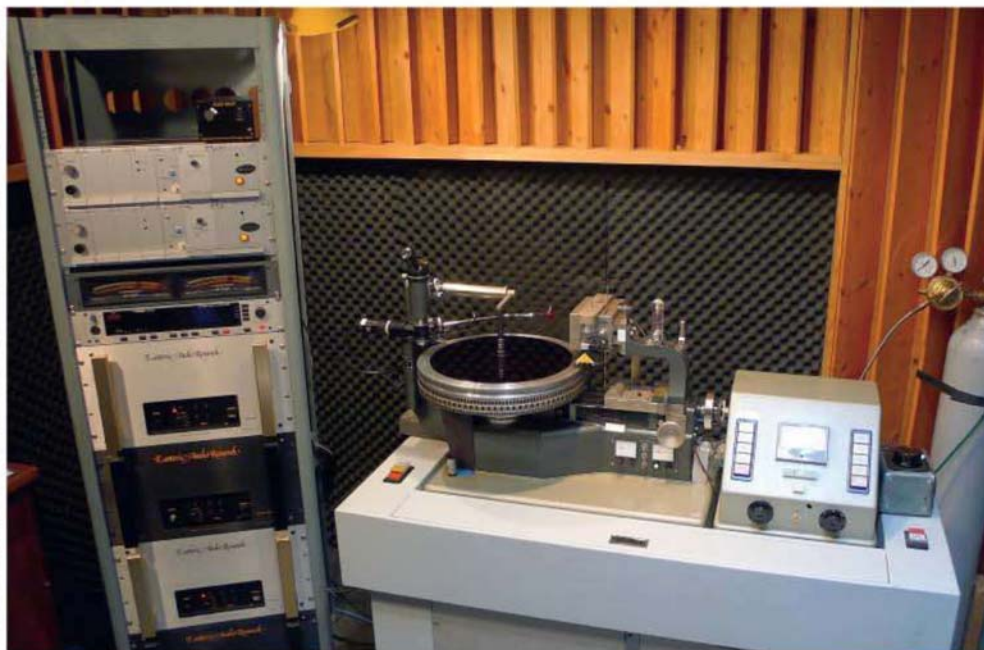
ABOVE: Mobile Fidelity Neumann VMS70 mastering lathe with EAR electronics controlling the cutting head
