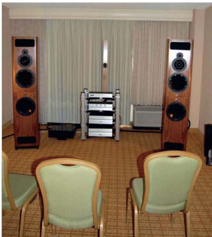
Listeners were blown off their chairs by PMC's MB2 XBDi tower speakers! Developed from an active studio monitor, the design features two 310mm woofers and external crossovers. Source was a Bryston BCD-1 CD player, feeding a Bryston BP26 preamp and two 7B SST monoblocks. See www.pmc-speakers.com .
