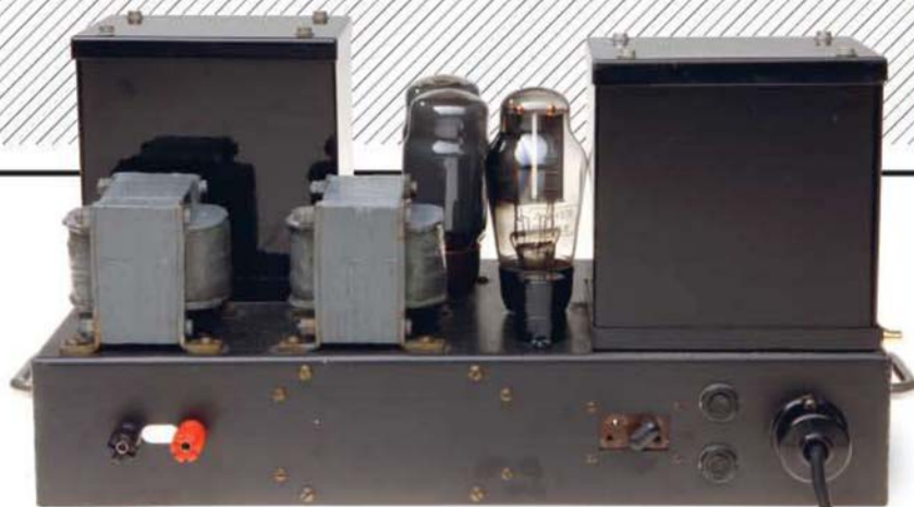
ABOVE: The Partridge o/p transformer's 8ohm secondary tap is terminated here in a pair of 4mm speaker posts. Note the three-pin Bulgin-style mains plug!
