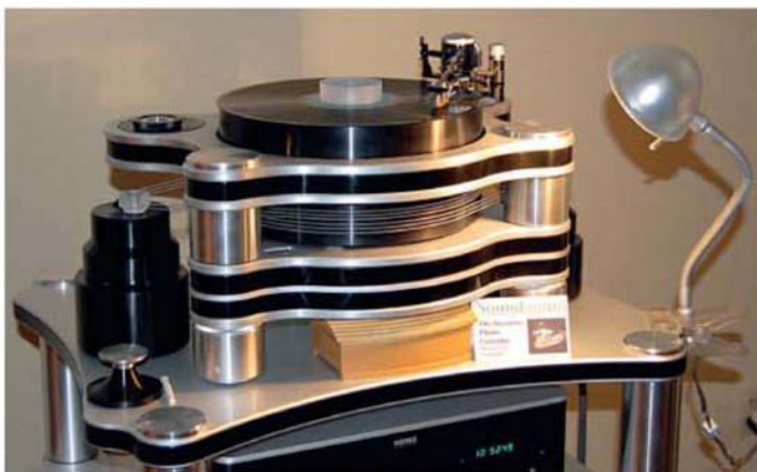
The Hanss Acoustics T60 turntable, designed in Germany with parts made in China. It features a magnetically suspended 200mm-deep aluminium platter driven by two AC motors via six silicone rubber belts. The solid base is of sandwiched aluminium and acrylic. The tonearm is the Triplanar VII with a Soundsmith Sussurro low output cartridge. See www.hanssacoustics.com .
