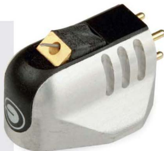
ABOVE: The Legacy moving-coil has a magnesium alloy body threaded for hex-drive fixing bolts; generator coil wiring is high purity copper and the stylus profile is Namiki Vital
