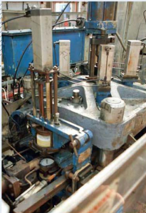
ABOVE: EMI Type 400 press is 1960s vintage; stamped records are inserted into inner sleeves (right)
