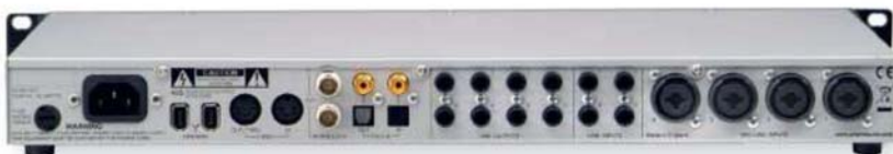
ABOVE: Packing eight balanced analogue inputs and the same number of balanced analogue outputs into a small back panel has meant that quarter-inch jack connectors are used. Optical and coaxial S/PDIF in and out are also provided
