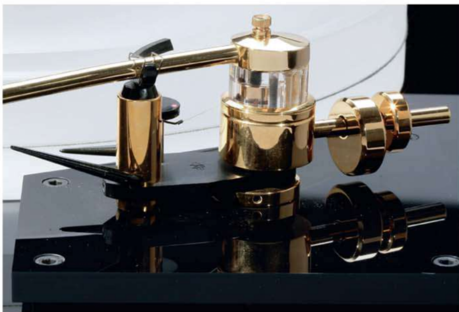
RIGHT: Seen here in gold-plated finish but also available in chrome, Mørch's DP-6 tonearm combines ball-bearings for lateral rotation with a double point bearing for vertical movement
