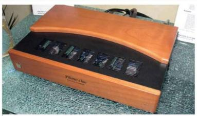
With all that wood, it had to be Unison Research. The Phono One contains five ECC83s, operating in Class A mode. Settings accommodate cartridges with 20, 47, 100 and 47kohm impedance requirements, with capacitance adjustable in four levels from 100 pF-420 pF. www.unisonresearch.com.
