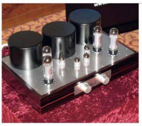
WLM Acoustics' Sonata is a tube product that makes me want to convert transistor users, for it screams 'classic': four EL34s in push-pull array is claimed to deliver a useable 2x20W in Class A mode, or 2x35W in Class AB. www.wlmacoustics.com.
