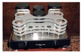
Mastersound's Evolution 845 is a single-ended stereo amp using four of my favourite tubes, the source of its nomenclature. Power is rated at 2x55W in pure Class A – and that's under-stressing the tubes. The rest of the tube line-up includes two ECC82s and two 6SN7s. www.mastersoundsas.it.
