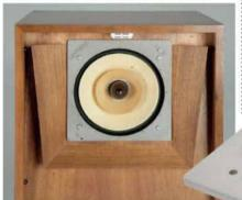
ABOVE: A Lowther PM6A driver pictured in situ and (right) the driver itself; power handling was a claimed 20W and impedance 15ohms
