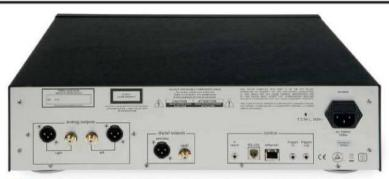
ABOVE: As befits a product of this class, both analogue and digital outputs offer a choice of unbalanced connection via phono sockets or balanced connection via XLRs. Various control interfaces are also provided for installed systems
