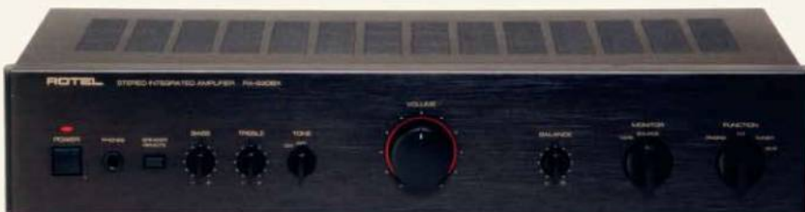
ABOVE: A huge hit from 1994 – Rotel's RA-930BX, rated at 30W but delivered 50W
