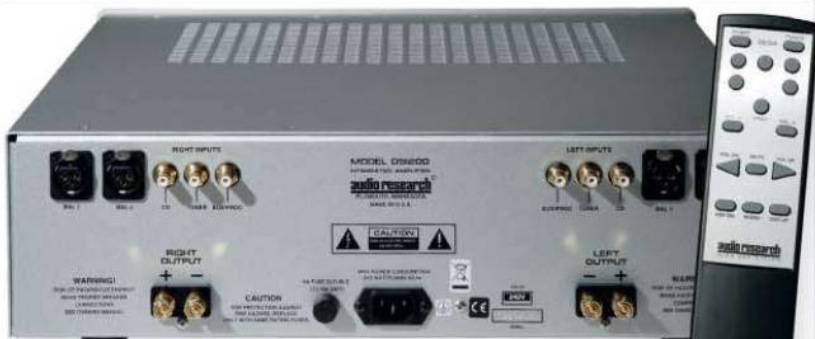
ABOVE: Three unbalanced (RCA) and two balanced (XLR) inputs are joined by single sets of speaker binding posts (the 4mm sockets are sealed). Full remote control over inputs, options and volume is included
