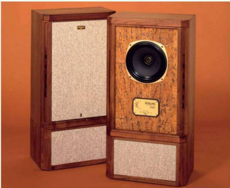
LEFT: Tannoy Stirling model from the 1990s sporting a 10in Tannoy Dual Concentric driver
