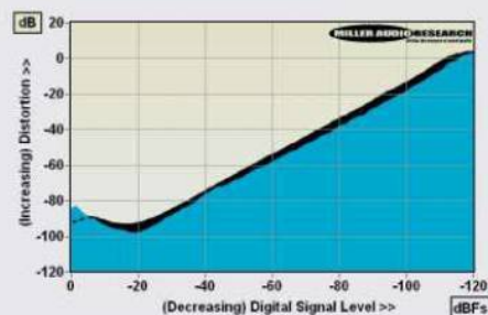
ABOVE: Distortion versus digital signal level over a 120dB dynamic range using 24-bit data at 1kHz (black) and 20kHz (blue)
