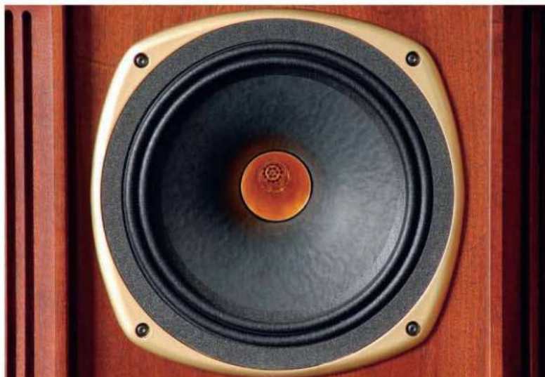
ABOVE: A 10in dual concentric driver housed in a Tannoy Kensington cabinet; at the heart of the doped paper pulp bass driver sits a 2in round-wire wound voice coil
