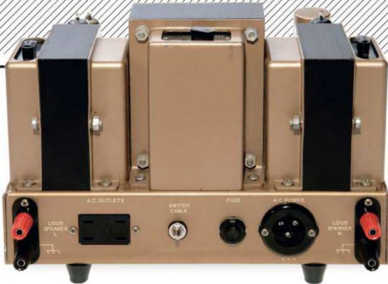
ABOVE: The 4, 8 and 16ohm speaker taps are configured via a link at the top of each transformer, leaving a single set of binding posts at the rear (uprated in our sample)
