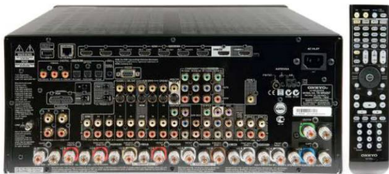
ABOVE: Comprehensive connectivity trumps the competition with eight HDMI's (one on the front) but far fewer analogue and S/PDIF inputs and outputs. The Universal port supports Onkyo accessories such as various iPod docks and a DAB+ module.
