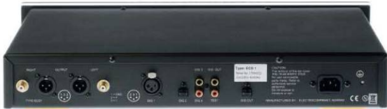
ABOVE: Plenty of connections on offer with one optical and two coaxial S/PDIF digital inputs joined by an AES/EBU (XLR) option. There are coaxial and optical digital outputs as well as both single-ended (RCA) and balanced (XLR) analogue outputs
