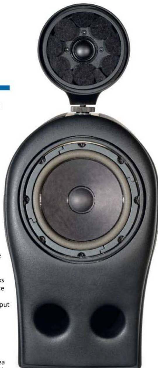
ABOVE: Both drive units are covered by a thin foam 'grille' which are pushed into a circular groove within the cabinet moulding. A metal trim ring is then added to disguise the groove
