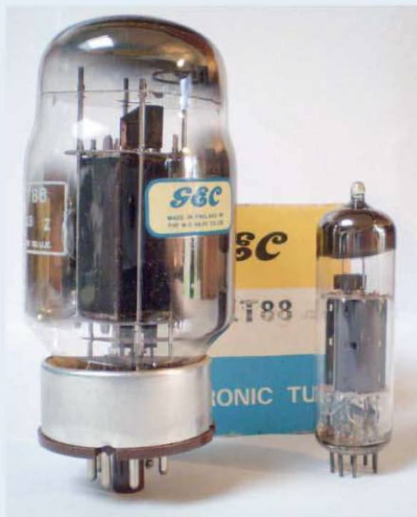
BELOW: Little and large – two popular 1950s power valves in the form of a GEC KT88 beam tetrode with box (left) and an EL84 output pentode
