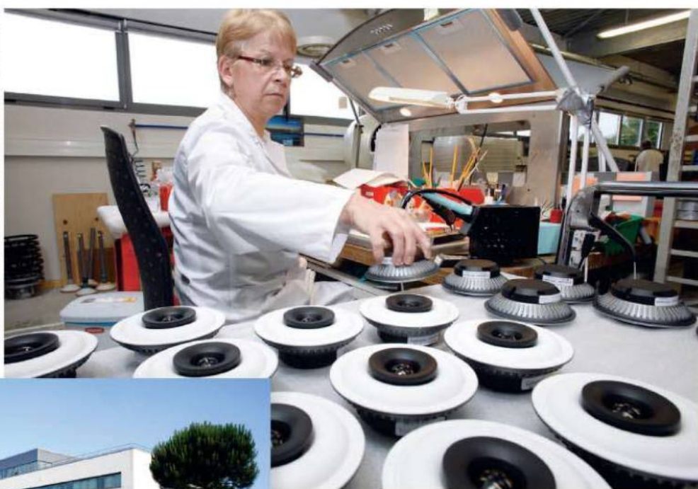
ABOVE: Josiane hand assembles and tests a batch of BC13 drivers, coaxial units with aluminium frames and magnets used in three-way Cabasse models such as the Iroise, Egea and Bora
