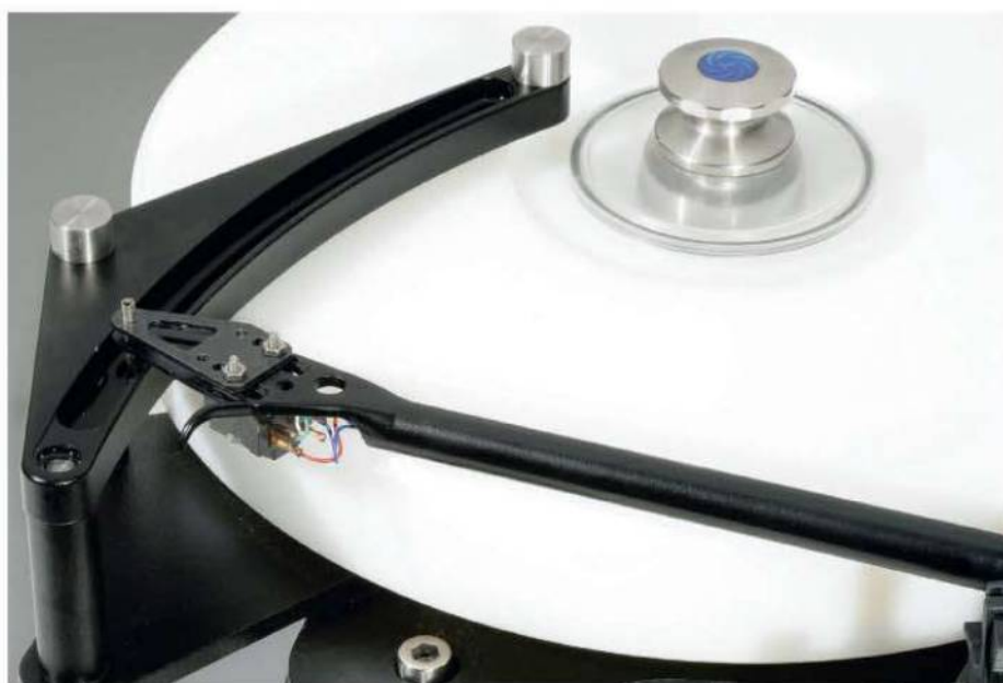
ABOVE: Paddle glued to an outrigger sits in a trough of silicone to provide damping of arm/cartridge resonance. Clear plastic record clamp allows reading of the label
