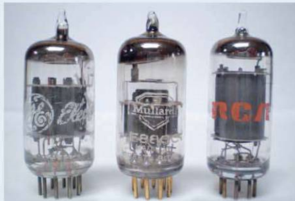
ABOVE: 12AU7 (ECC82) double triode from General Electric's 12A...7 series (left); Mullard E88CC double triode from 1958 (middle); RCA 6BJ6 pentode (right)
