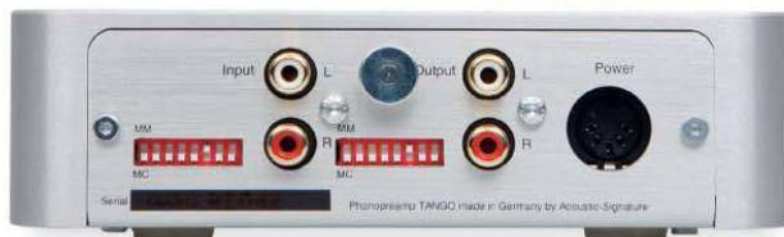
ABOVE: Along with phono in/outs and a DIN socket for power input, a set of DIP switches for each channel set load impedance (MC) and capacitance (MM)
