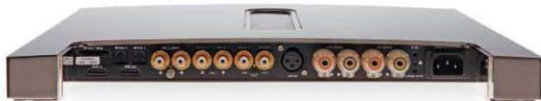
ABOVE: Devialet has equipped its amp with an HDMI v1.3 input and output, two Toslink optical digital inputs (up to 24-bit/192kHz) and a balanced AES/EBU digital input. The MM/MC phono and line input, two coaxial digital inputs/outputs (up to 24-bit/192kHz) may be configured to use any of the six visible RCA sockets.
