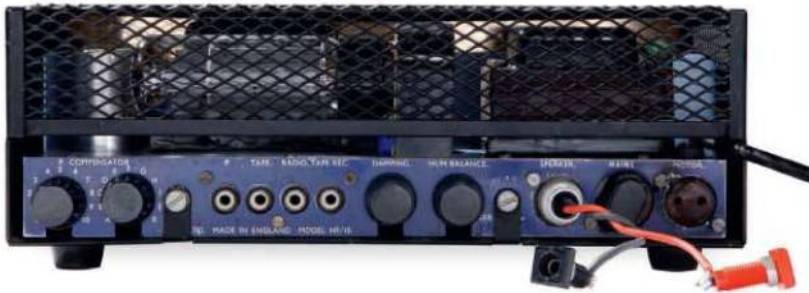
ABOVE: Mono radio, tape and phono inputs were provided alongside 'Dialomatic' pickup compensation (left). Our sample is modified with flying 4mm speaker connections but note the 'Hum Balance' and output impedance 'Damping' controls
