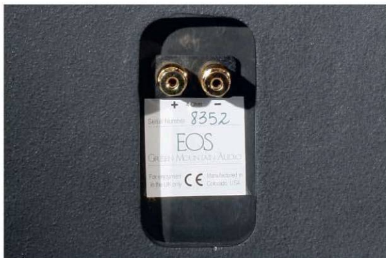
ABOVE: The moulded enclosure, cast using a mineral-loaded resin, facilitates a curved cabinet form that benefits both acoustic and structural performance. The crossover and single 4mm cable terminals are held in place with a rubberised glue
