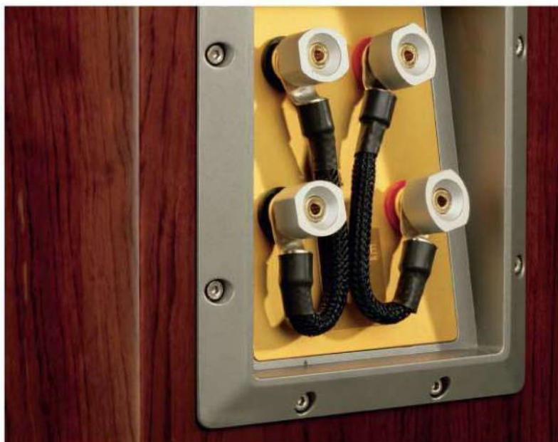
ABOVE: A split crossover allows for bi-wiring or bi-amping, the upper pair of terminals connecting to the mid and treble sections and the bottom pair to the bass
