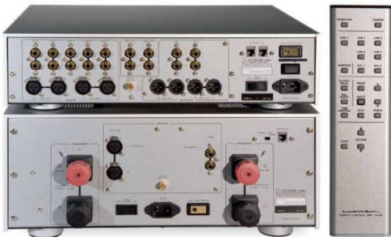
ABOVE: Faultless ingress/egress for both, with superbly made connectors, XLRs for balanced, indication of AC mains polarity, and, on M-600A, huge speaker terminals. Remote covers every function, including preset access
