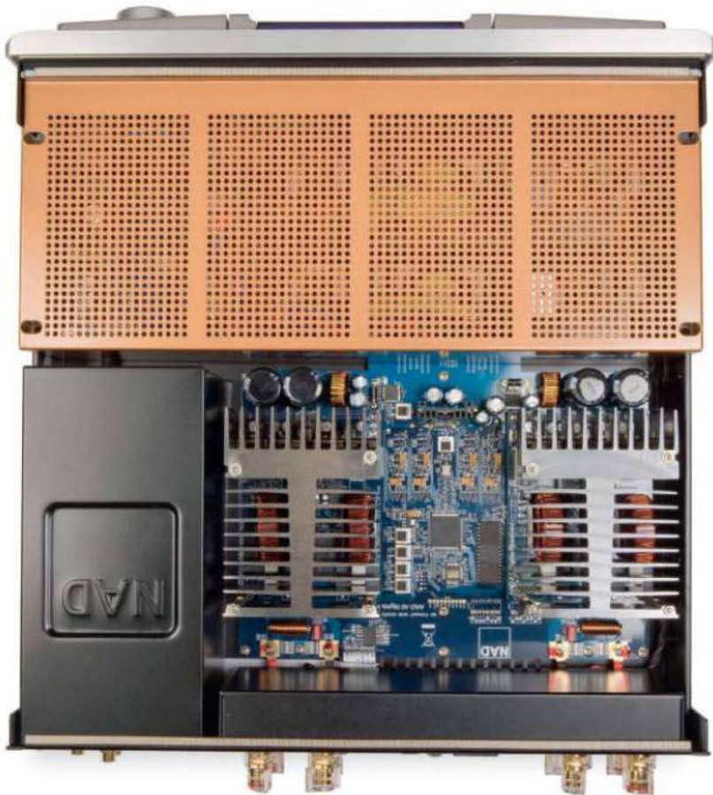
ABOVE: Inside the M2 which employs separate switchmode power supplies for the input and modulator stages plus each of the L/R MOSFET output switching stages
