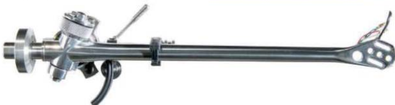
ABOVE: Single-piece arm tube and headshell with finger lift is highly-polished aluminium, with no coating applied in order to keep mass to a minimum
