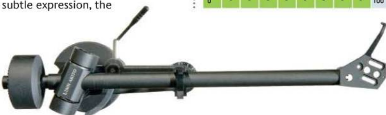
ABOVE: Sturdy pressure die-cast headshell featuring a practical finger lift is pinned and glued to the Akito's straight-profile single-piece alloy arm pipe
