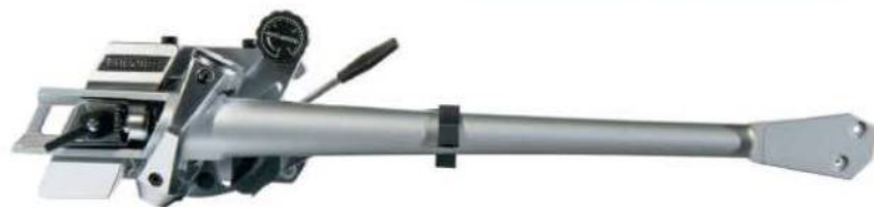
ABOVE: One-piece pressure die-cast tapered magnesium arm pipe is internally damped. Anti-skate/bias compensation is by a tension spring and calibrated dial
