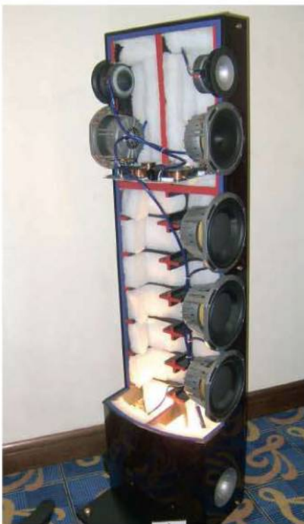
Triangle had an awesome set-up in a huge room, using the biggest Emille valve amps to drive its flagship Grand Concert speakers. Also from the French maker's Magellan SW2 range is the Concerto, seen here as a cutaway. www.triangle-fr.com .
