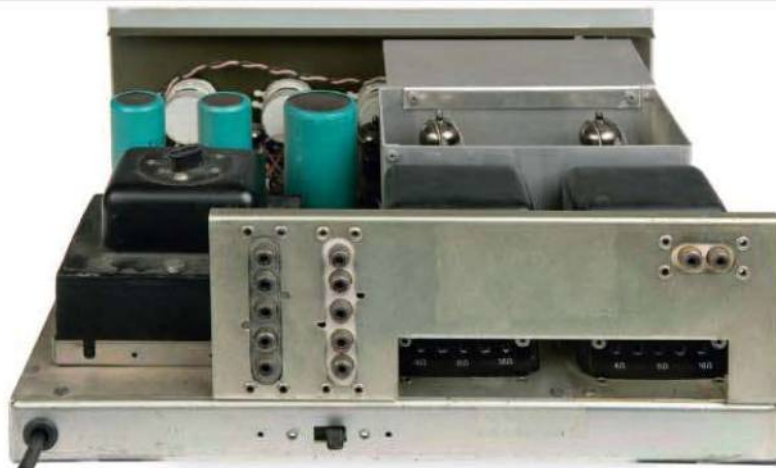
ABOVE: Inputs for ceramic/crystal pick-ups (phono), tape (in/out) and radio are offered while three transformer taps are provided for 4, 8 and 16ohm speaker loads
