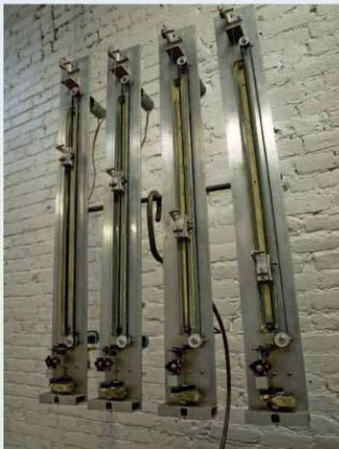
BELOW: A single guitar bot – four individual strings, each with a moving bridge
