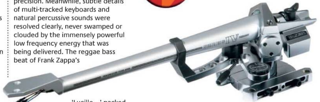
ABOVE: Clamp bolts on the base release the arm for both horizontal and vertical adjustment. Underslung counterweight is a tungsten-alloy block suspended on a damped suspension
