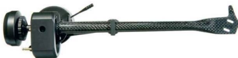
ABOVE: Single-piece carbon fibre arm tube, its conical profile designed to avoid standing wave reflections, morphs into headshell. Bias is via thread and weight
