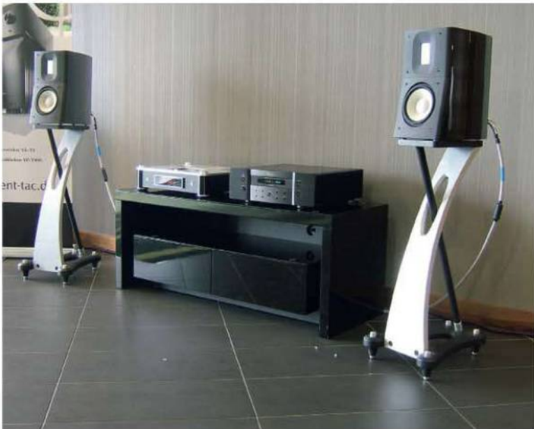
A real eye-catcher was this combination of TAC C-80 player and Vincent SV-234 amp, with Raidho Ayra C1.0 speakers on their own dedicated stands. These slick Danish mini-monitors use a 115mm ceramic-cone bass/mid driver, reflex loaded by a rear port, matched to Raidho's own ribbon tweeter. www.mv.audio.co.uk , www.duodistribution.co.uk .
