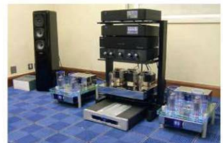
Valve amp specialist Art Audio showed off the new Conductor preamp, designed to do justice to its latest single-ended power amps, with a direct-coupled DC servo eliminating output capacitors. It's seen here with Vinyl 1 phono stage, Diavolo single-ended 300B stereo power amp and a pair of the mouthwatering Adagio monoblocks, each using two 520Bs, single-ended in parallel. CD source was a PS Audio transport and DAC while speakers were Ars Aures Mi from Italy. www.artaudio.co.uk .
