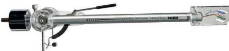
ABOVE: Anti-skating/bias is via thread and weight. The hole through the counterweight is offset, consequently rotating it alters cartridge azimuth
