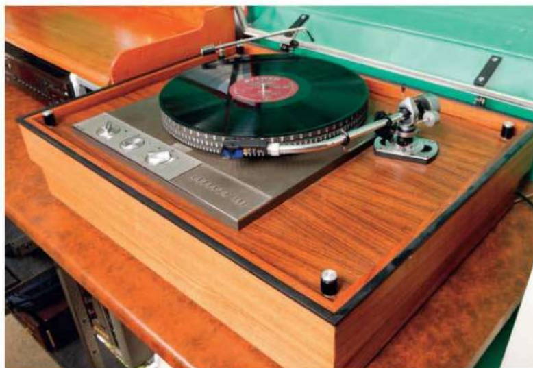
RIGHT: Garrard 401 deck in its SME plinth, with 3009 arm and Ortofon MC20 cartridge; a Philips CD624 player can be seen to the left
