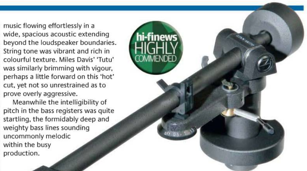
ABOVE: Conventional design with anti-skate/bias compensation provided by a tension spring and dial, while the pillar can be raised/lowered in the arm collar to adjust VTA
