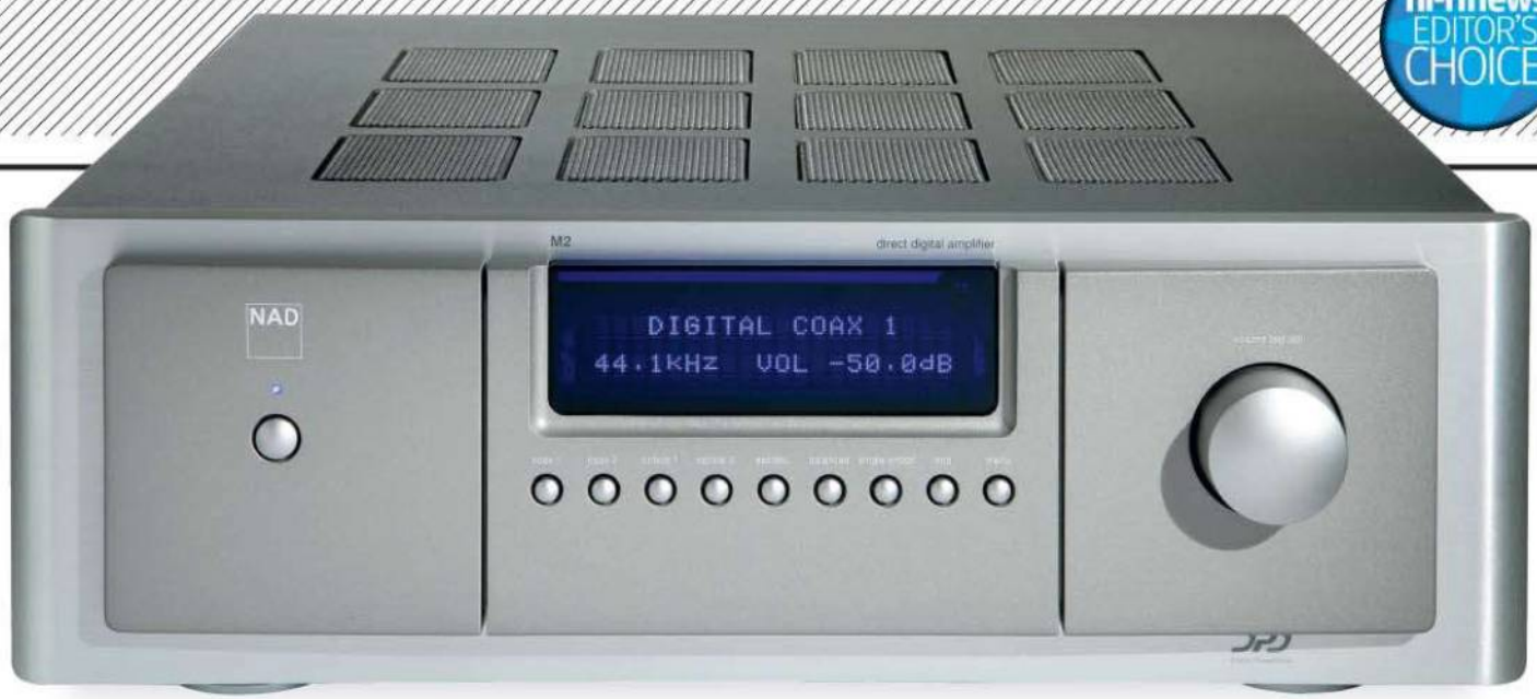
ABOVE: The selected input and (for digital sources) incoming sample rate is indicated on a bold display. The volume/setup control operates from -70dB to +10dB in 0.5dB steps
