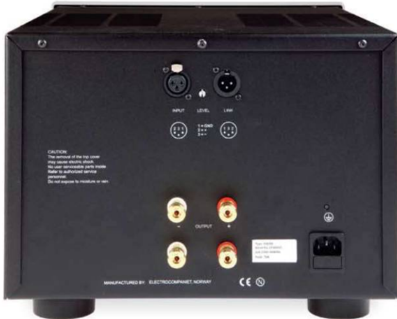
ABOVE: A balanced (XLR) input sits alongside a link output for daisy-chaining amplifiers. Input level adjustment provides for level matching in bi-amped systems
