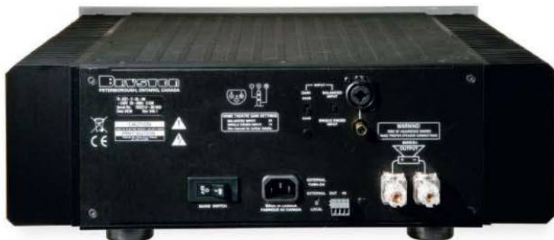
ABOVE: As usual with Bryston amplifiers, input connection is either balanced via XLR or unbalanced via phono and input sensitivity is switchable by 6dB. The terminal block connector by the mains socket provides for remote switch on/off
