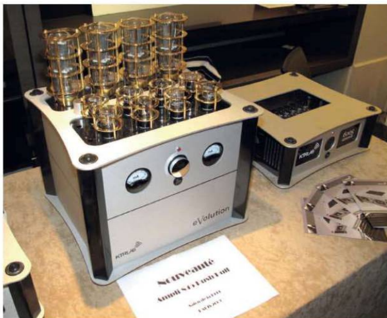
KTR Lab's 845 Push-Pull is a beautifully-constructed, single-chassis stereo power amp using a pair of 845s per channel, as the name says, in push-pull mode. Like Rolls-Royce, KTR, on this occasion, is averse to revealing the power. Also on the stand was a CD player matching the styling of the electronics, but again KTR Lab was saying nothing. www.ktr-lab.com .
