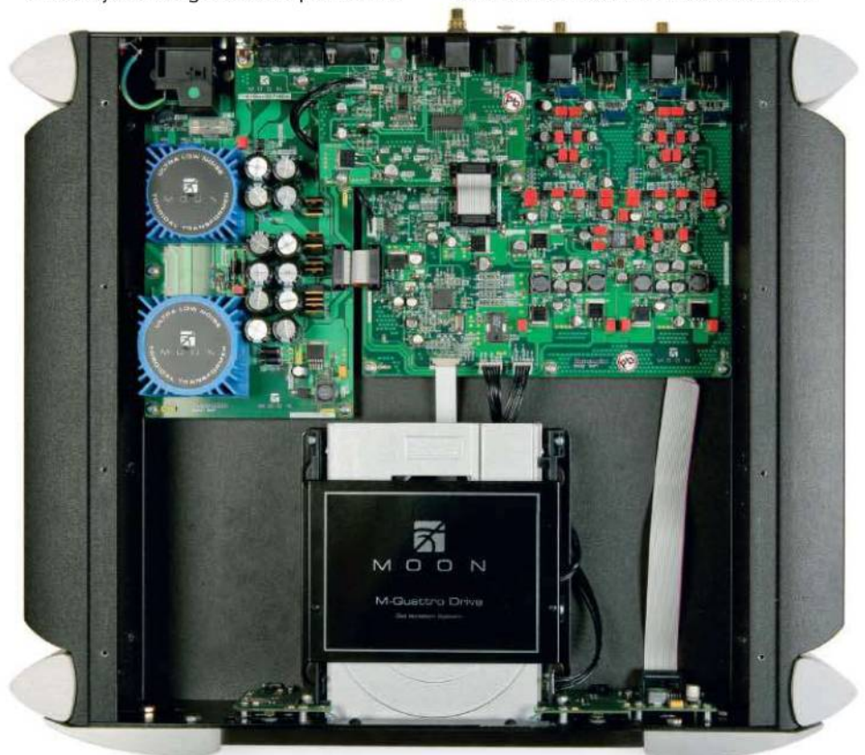
RIGHT: Uncluttered internal layout and the substantial casework help keep operating temperatures low to the benefit of reliability. An optional outboard power supply is on its way
