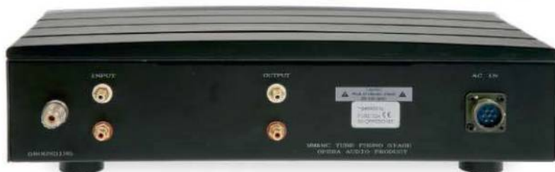
ABOVE: Rear panel carries a single pair of inputs switchable for MM or MC, a pair of outputs and a multi-pin connector for the outboard power supply
