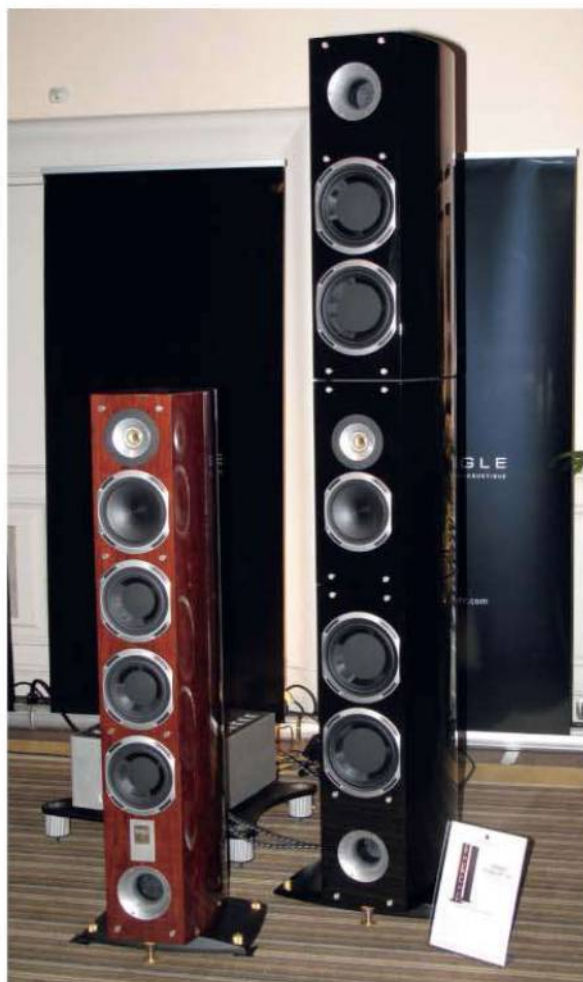
Triangle's Grand Concert SW2 – the tall, black speaker – is a bass-reflex three-way divided into sections housing two tweeters, two mids and four woofers, with ports top and bottom. The maximum output is a fearsome 116dB/1m, from a model with only a middling 91dB/1W sensitivity. www.triangle-fr.com .
