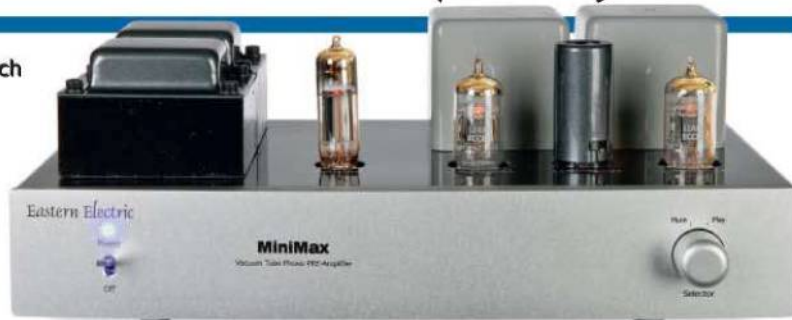
ABOVE: Carrying the smallest signals, the first-stage tube is the most sensitive to disturbance and so is shielded
