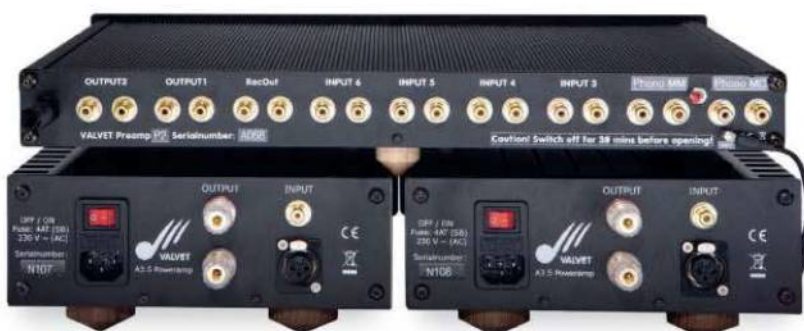
ABOVE: Rear view of Valvet's flagship system shows clear layout and superb access to all socketry but also emphasises an anomaly: why do the power amps accept balanced inputs, but the preamp is single-ended only? Note hardwood coned feet
