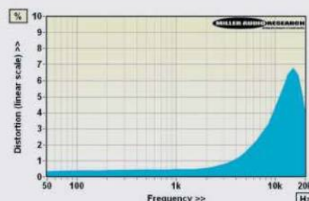
ABOVE: Tracing and generator distortion (2nd-4th harmonics) versus frequency from 50Hz-20kHz (-8dB re. 5cm/sec). This is fine result
