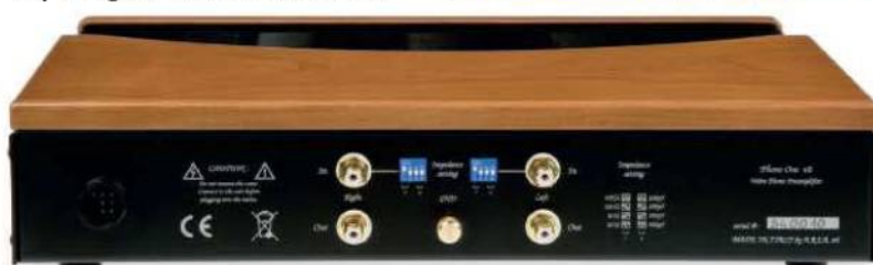
ABOVE: Input sensitivity is fixed but DIP switches give load impedance settings of 20, 50, 100ohm or 47kohm, or add capacitance loading of up to 470pF
