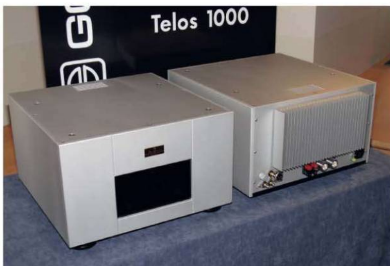
Goldmund's Telos 1000 is a monoblock said to deliver a kilowatt into 4ohm, requiring 16 separate power transformers. Features include an internal D/A converter, full DC and output overload protection, balanced and unbalanced analogue input with level adjustment and RCA digital input and output with 96kHz/24-bit capability. Dimensions are 440x495x280 (wdh), weight is 70kg, and price is, er, high. www.goldmund.com .
