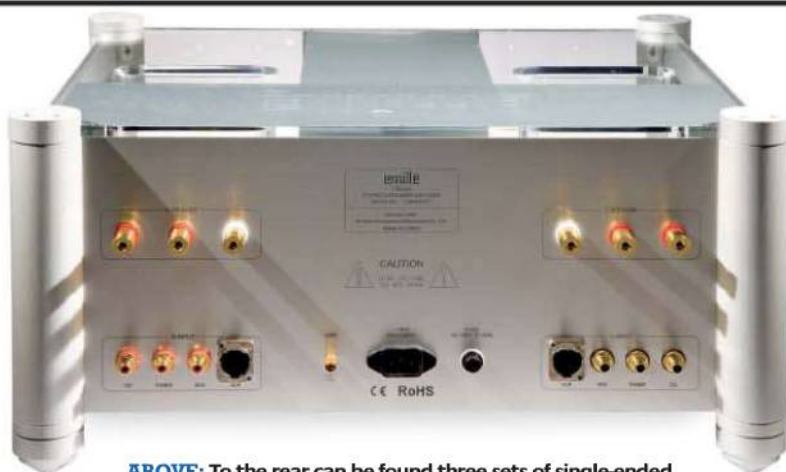
ABOVE: To the rear can be found three sets of single-ended RCA input sockets together with a balanced input pair (XLRs); meanwhile, the speaker terminals are gold plated and offer both 4 and 8ohm taps
