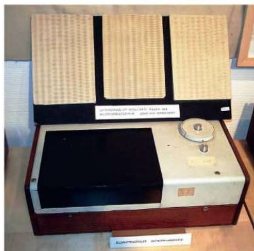
ABOVE: Design prototype of a player for the Telefunken TeD video disc, first announced in June of 1970, alongside Decca promotional material from July 1970, which shows the finished product
