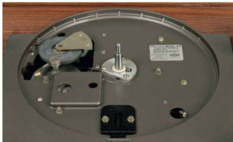
ABOVE: The cast chassis is what helps give the Garrard 401 its clean, fast sound, along with the jewel-like idler drive system. Note the mechanical brake to the right
