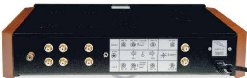
ABOVE: The extra pair of phono sockets is for plug-in resistors which adjust MC load impedance. When none are fitted, as here, the load is 47k ohms
