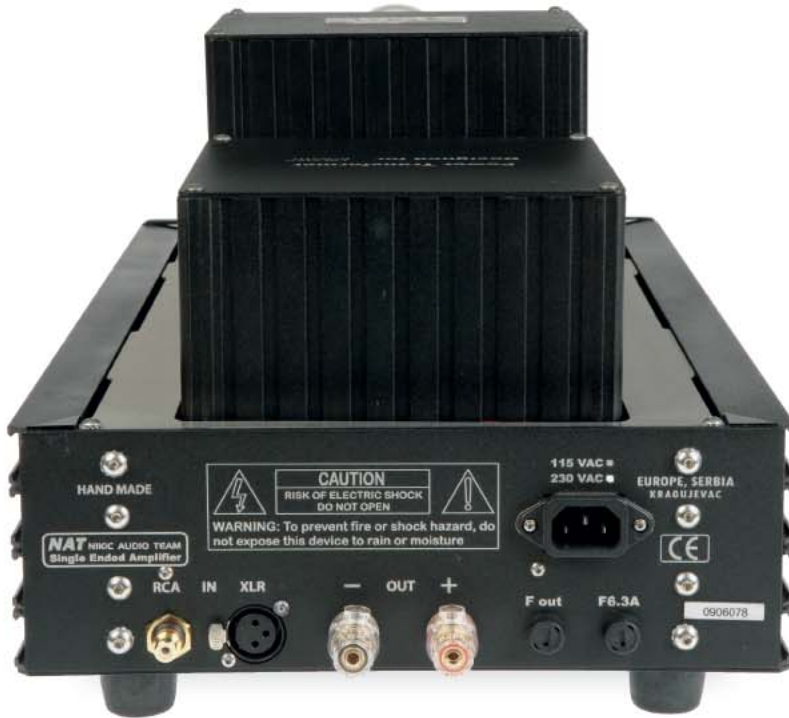
ABOVE: Both RCA and XLR inputs are single-ended while the single 4mm speaker output posts are coupled to both 8ohm and 4ohm transformer taps via a front switch
