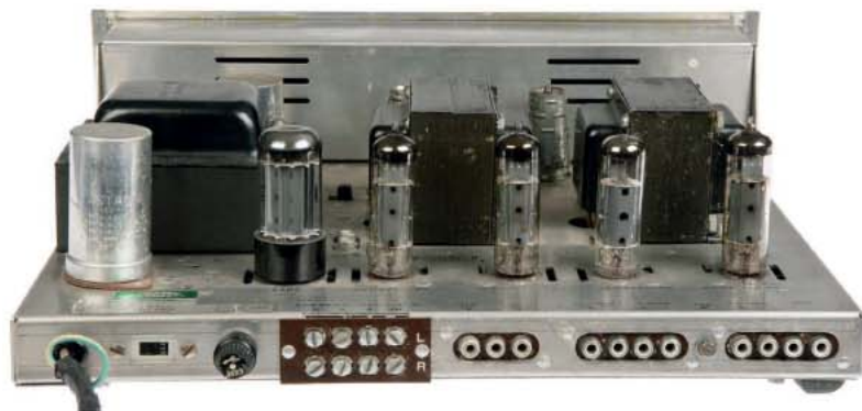
ABOVE: The rear of the Scott (l-r) - supply voltage switch; removable fuse; set of multi-tapped 4, 8 and 16ohm speaker outputs; centre channel output, left and right outputs; tape in and tuner in; ground terminal; inputs for ceramic cartridge and MM
