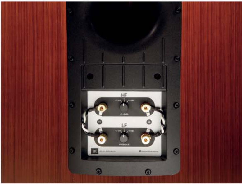
ABOVE: Bi-wire/amp input terminals, plus HF and Presence controls for fine tuning. Cover plate above hides a switch to disable the crossover for active drive
