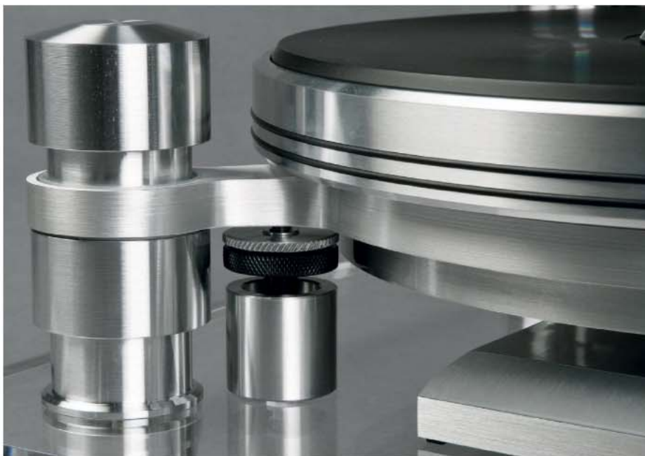
RIGHT: By each suspension tower a cup of silicone fluid and adjustable plunger (with locking ring) provides damping of the subchassis
