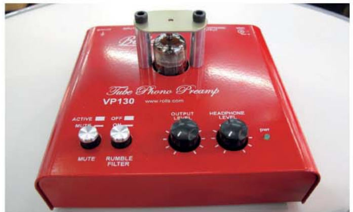
Bellari's bargain-basement VP129 valve phono preamp has been replaced by the $250 VP130 with a new switching power supply to accommodate 100-240V. That means we can order 'em from the USA without reservation! Tube is a 12AX7, and it'll drive headphones too. www.musicchallaudio.com .
