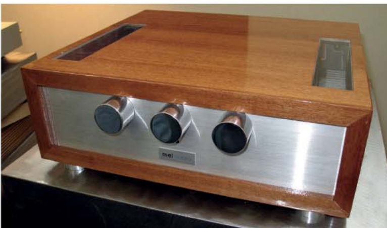
As a rule, Mel Audio opts for the futuristic, but the Kana is pure retro. Shown in prototype form, this new integrated amp from Italy is dual mono and solid-state, yielding 2x50W and able to accept five sources. Phono is an option. www.melaudio.it .
