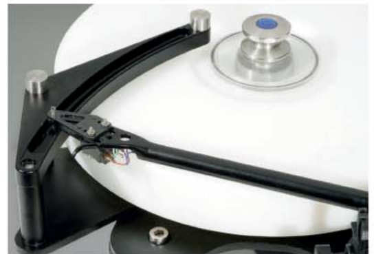
ABOVE: Townshend Rock 7E with paddle in trough of silicone to provide damping of arm/cartridge resonance
