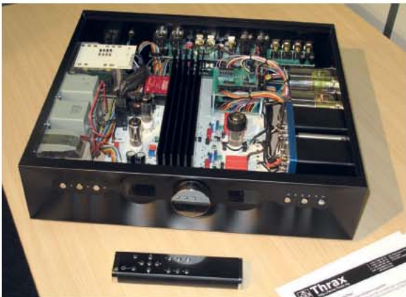
From Thrax, a fascinating line level tube design that accepts four unbalanced and two balanced sources. The amplification stage is a single indirectly heated triode while the case is fashioned from aircraft-grade aluminium. Price is €15,000. www.thrax.bg .
