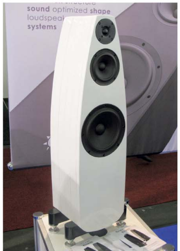
Emme's Beta contains an 8in woofer in its tapered, sandwich construction enclosure. Sensitivity is 88dB. Also available is the similarly-shaped Gamma with 12in woofer. www.emmespeakers.com .
