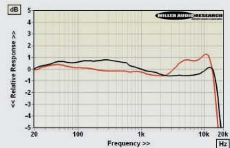
ABOVE: Left (black) and right (red) frequency responses, lateral groove modulation at -8dB re. 5cm/sec. Flat to within ±1dB up to 15kHz
