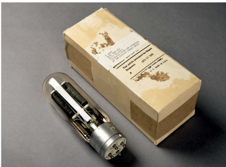
RIGHT: The heart of the amp – a direct-heated 211 triode tube from General Electric and 'packaged under the direction of the Chicago Signal Depot' on April 30th, 1945
