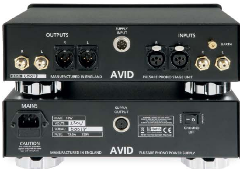
ABOVE: Single-ended RCA inputs and outputs are joined by balanced inputs and outputs. There's a ground lift option on the PSU if you encounter a hum loop
