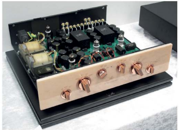
Audio Exklusiv's P7 valve preamp was seen with a selection of beguiling front panel options. The unit is dual-mono, with short signal paths for four line level sources plus tape. An MM or MC phono board is an optional extra. www.audioexklusiv.de .
