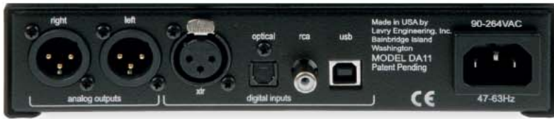
ABOVE: Don't panic: Lavry supplies XLR-to-RCA adaptors for driving preamplifiers or power amps without balanced inputs. The four inputs are digital-only
