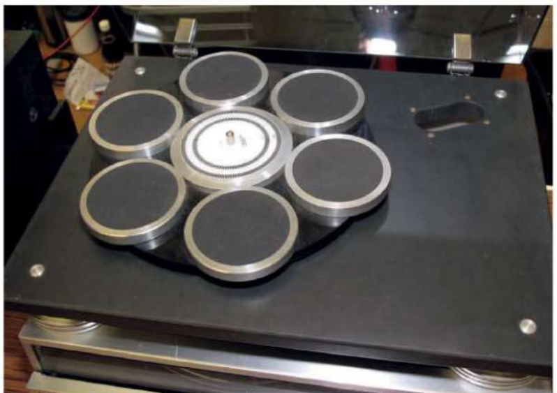
One of the most controversial turntables of the Great Turntable Wars of the 1970s and 1980s, this direct drive JBE featured a slate plinth and silent running. The model on offer had an SME cut-out and a price of only £250. Its condition was excellent, with even the dustcover being in great shape.
