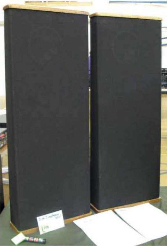
More rare Americana, a pair of DCM Time Frame TF-350 loudspeakers, smaller sisters to the iconic Time Windows. These were floorstanders sold in mirror-image pairs, with each enclosure containing a 6.5in woofer and 3/4in tweeter, in a chassis standing 38in tall, with a footprint of 15x6in. Part of the design included foam covering for the surfaces beneath the cloth pullover sleeve. The DCMs were known for their freedom from boxiness, and £110 for the pair seemed like a painless punt to me! (I'd have loved to match them with the Rappaport...)
