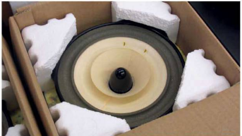
An unused pair of Lowther drivers is enough to cause palpitations amongst any gathering of anachrophiles with a penchant for DIY cabinetry, as did the UK-made horns seen at Bracknell. Shown is one of two still-in-the-box, utterly new and virginal PM2Cs, an 8ohm model good for 98dB/1W!
