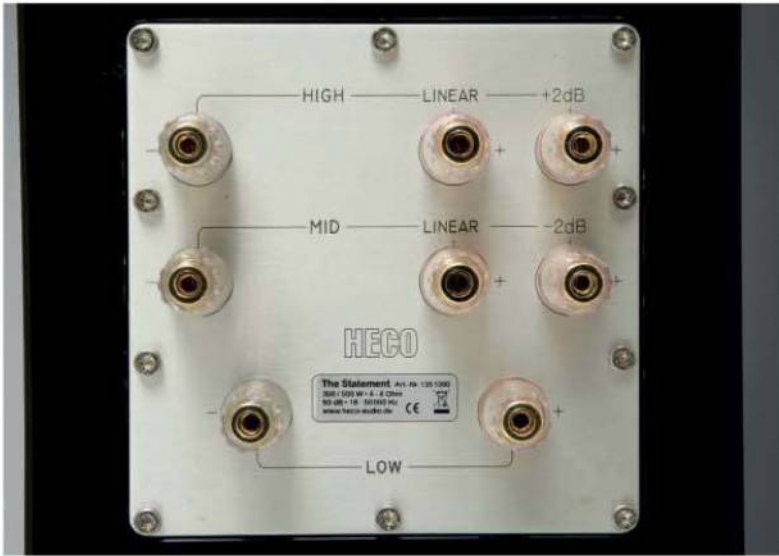
ABOVE: Split crossover allows bi-/tri-wiring or bi-/tri-amping, and includes separate positive terminals for lowering midrange or boosting tweeter output by 2dB
