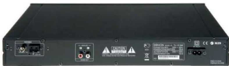
ABOVE: Rear panel fittings are standard, except that the mains input is via a 'figure of eight' two-pin connection, rather than the more usual IEC receptacle
