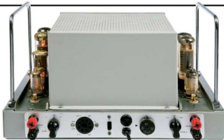
ABOVE: All controls and settings offer easy access, including the loudspeaker impedance selector, mains switch and voltage taps. The phono input sockets are located close to the input valves in a bid to minimise noise and interference
