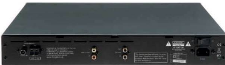
ABOVE: Extra phonos are for the My-Link comms bus, which can connect other Myryad components to give whole-system control via any one unit's IR receiver
