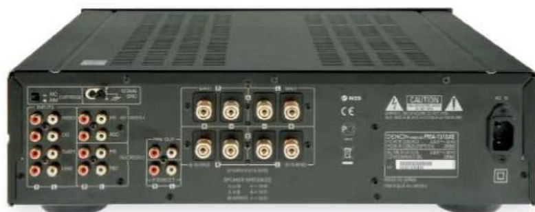
ABOVE: Five line inputs and two tape outputs are joined by a MM/MC phono input and pre-out/power-in sockets. The two sets of speaker terminals are not switchable
