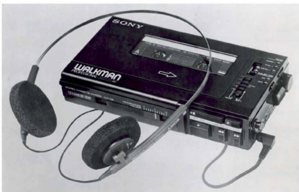
ABOVE: Original Sony WM-D6 with the supplied headphones – a far cry from ear-buds. The model name was changed to WM-D6C when Dolby C was added
