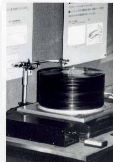
ABOVE: Not a multi-changer version but a demo of the powerful motor torque
