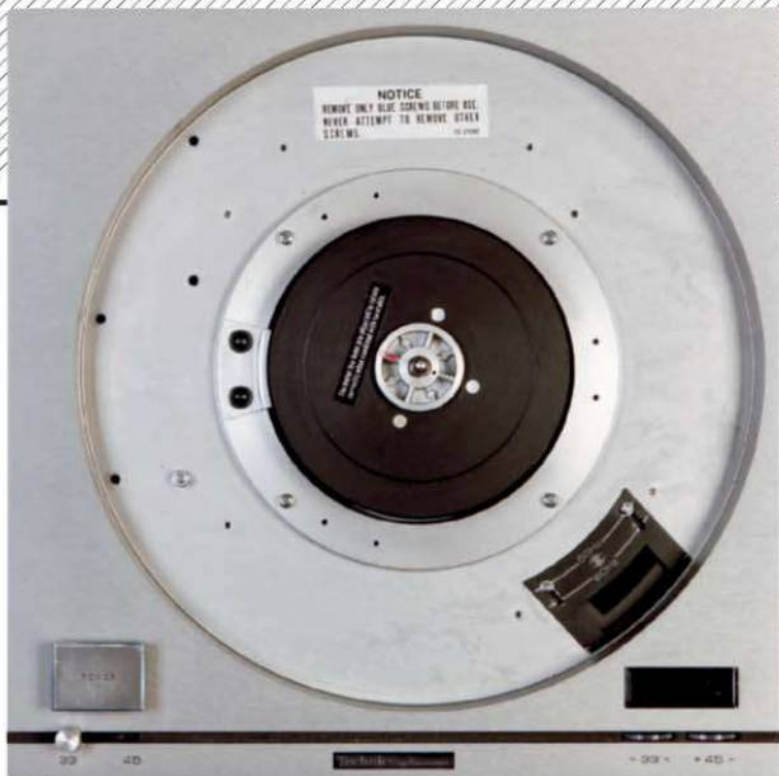
ABOVE: Plan view showing the thin-wall aluminium construction common to both the MKI and MKII decks. The decks' chassis were the same size
