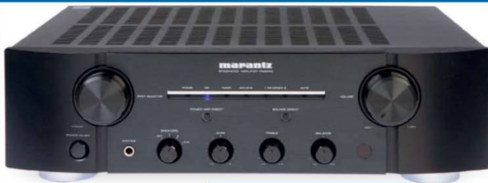
ABOVE: High feature count sees speaker selector on fascia together with Source Direct and Power Amp Direct
