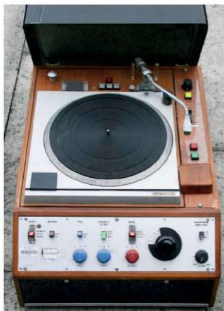
ABOVE: Fully specified BBC 'Gramophone Unit' based on the MKII and incorporating RIAA preamp, fader and BBC's own pantograph arm
