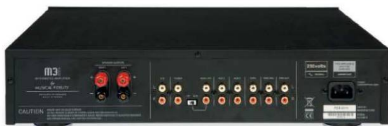
ABOVE: A single set of speaker terminals, with six line inputs – one of which can be switched to become a power amp in. Pre-out provides system upgrading flexibility
