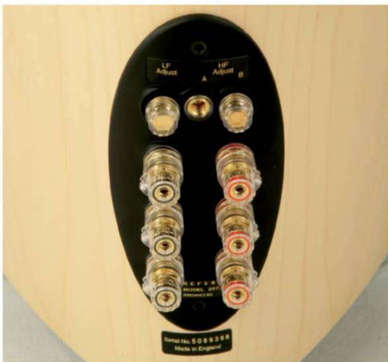
ABOVE: The crossover is split three ways to allow bi-wiring/bi-amping or tri-wiring. Bass and treble balance are both adjustable using threaded inserts
