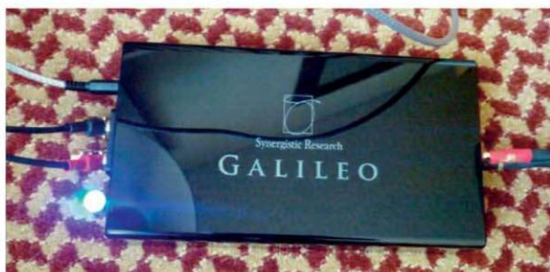
Synergistic Research's Galileo power supply provides DC bias to speaker cables in a bid to improve sound. Not found at CAS, despite an essay in the show guide, were LessLoss Blackbody spectral-energy dissipaters, said to minimize electromagnetic interaction among audio components.
