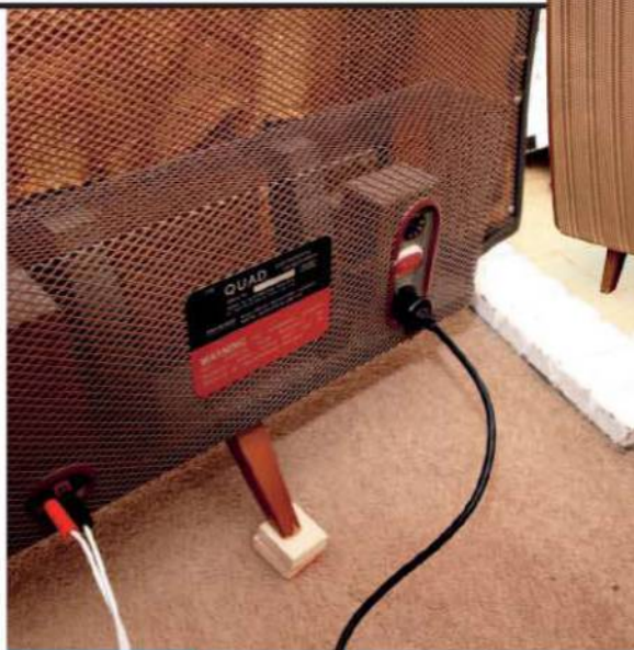
ABOVE: Late-production Quad Electrostatics are tipped forward slightly by small wooden blocks under the back legs
