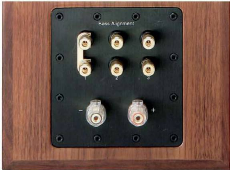
ABOVE: Single-wire binding posts are complemented by Teufel's bass alignment terminals that damp LF output depending upon which pair are bridged
