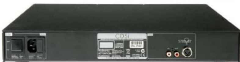
ABOVE: There are two single-ended analogue outputs via a pair of RCAs and a DIN socket, either or both selected via the remote handset; no digital output is provided
