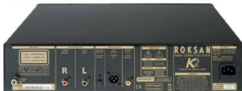
ABOVE: Analogue outputs are only single-ended RCAs, but unusually at this price there's an AES/EBU (XLR) digital out alongside optical and coaxial S/PDIF outputs
