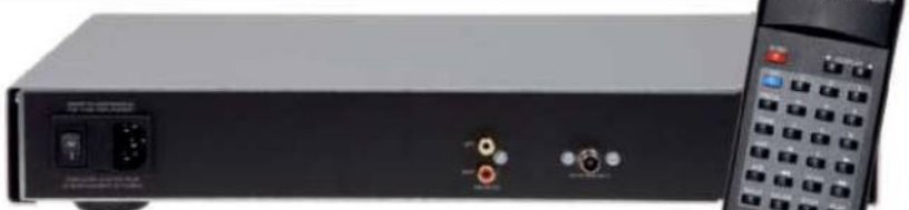
ABOVE: Rear panel has only the usual 75ohm aerial input and phono outputs plus power socket and switch. The many-buttoned remote will control a complete Micromega system
