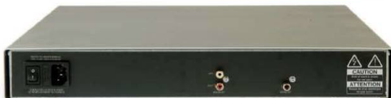
ABOVE: One set of single-ended (RCA) outputs and a coaxial digital output are all that's provided, although a DB9 connector can be fitted to allow RS232 control
