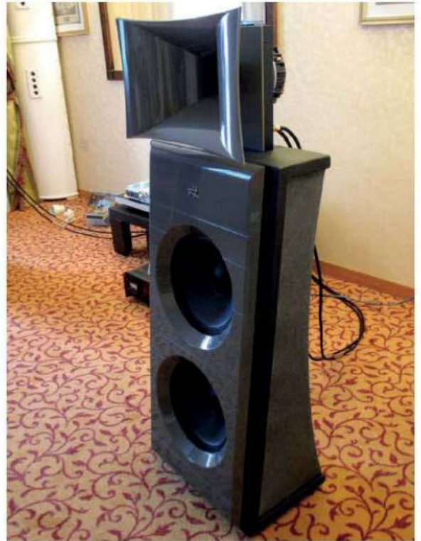
Diesis Audio's Caput Muni is a three-way system topped with a horn-loaded coaxial compression driver. Horn and baffle are made of Corian, contributing to a weight of 97kg for the 1370x512x365mm (hwd) structure. www.diesisaudio.com .
