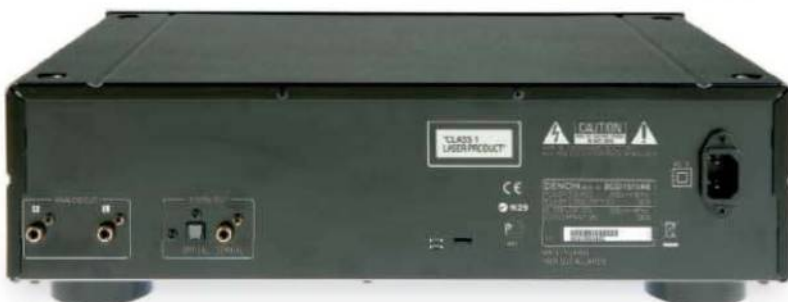
ABOVE: To the rear of the Denon can be found both optical (Toslink) and electrical (RCA) digital outputs alongside a pair of single-ended analogue outputs
