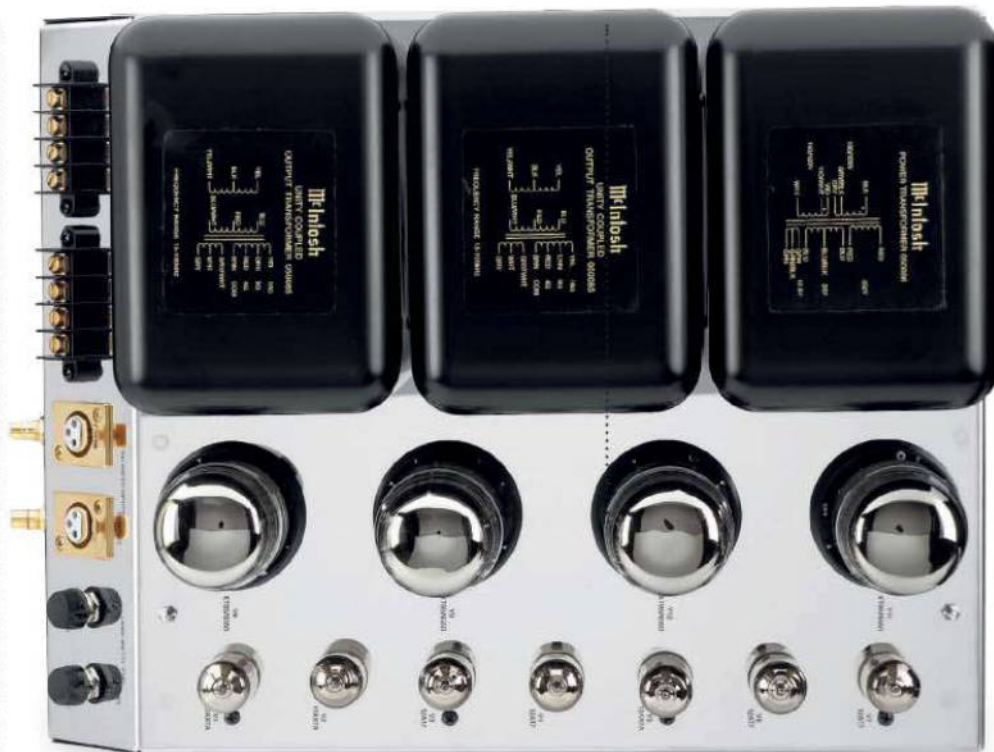
ABOVE: Top down view of the MC275 without its cage showing the four unity coupled output transformers, big KT88/6550 valves and smaller 12A27 and 12AX7 tubes
