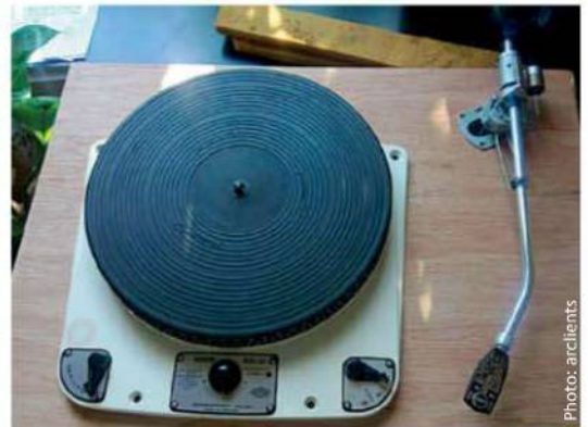
ABOVE: A Garrard 301 and SME arm ready to be bolted onto a brand new base, in this case made of laminated ply
