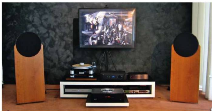
ABOVE: A pair of Emerald Physic loudspeakers on dem at the Raindrop Audio listening room in Singapore (see www.raindropaudio.com ); DSP processing allows for room acoustics correction
