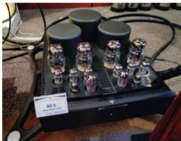
Balanced Audio Technology from the USA showed its flagship Rex monoblock (Balanced-Tube). Weighing 45.5kg, the all-triode, zero-feedback design delivers a claimed 160W at less than 3% THD using 6C33C-B tubes. Cost is a mighty £36,000 a pair. Ouch! www.balanced.com .
