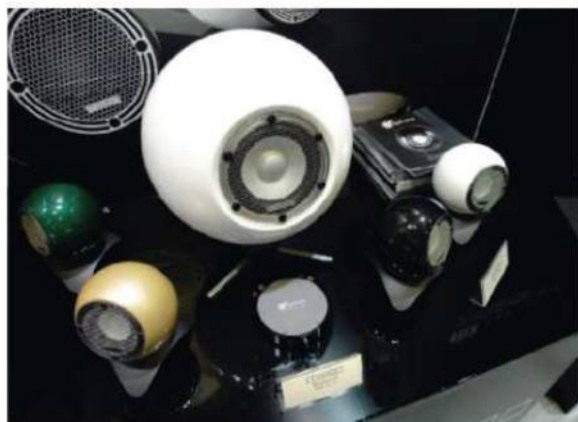
Mission used the event to show off its M-isphere 2.0 speaker range which comprises the M-isphere and M-isphere Mini, both available in eight colours. Each table-top enclosure houses a single driver and is powered by a separate Class D amp module. www.mission.co.uk .
