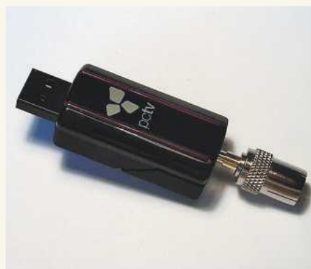
ABOVE: The Newsky TV28T TV tuner (left), which the author is using as a software-defined radio receiver, can be had for as little as £10 while the FUNcube Pro Plus (right) costs close to £200
