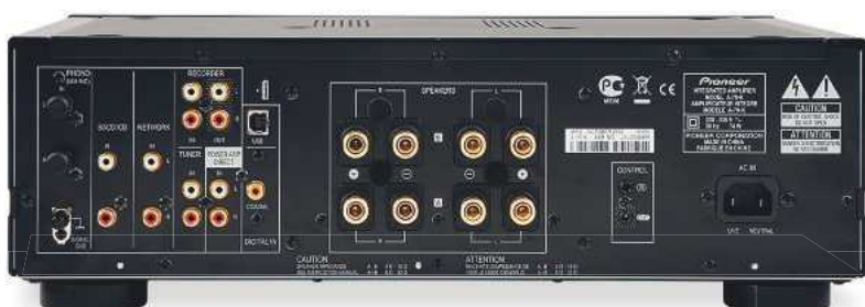
ABOVE: Two pairs of speaker binding posts dominate the back panel, along with USB and coaxial digital inputs and phono in, plus four standard RCA line inputs
