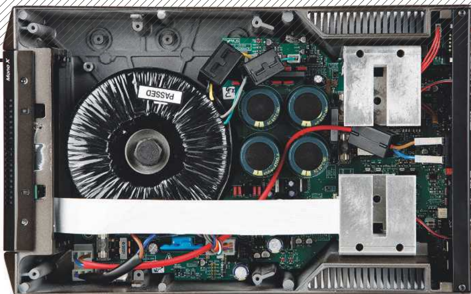
ABOVE: Inside the X 300 'zero-feedback' monoblock we see a 300VA toroid and a pair of devices for each supply rail mounted onto diecast aluminium heatsinking. The 'intelligent' fans kick-in at 58°C
