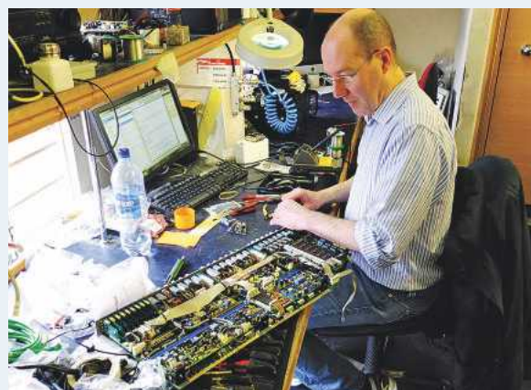
BELOW: In-house maintenance in AIR's workshop. Here engineer Paul Crowther is working on a channel section from the Studio 2 console
