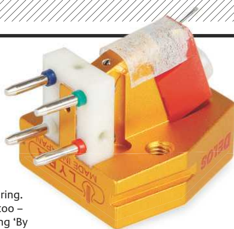
ABOVE: 2.5x75 \mu\text{m} Namiki line contact stylus and solid boron rod cantilever BELOW: Output pins are colour-coded and well spaced while the body has pre-tapped mounting holes
