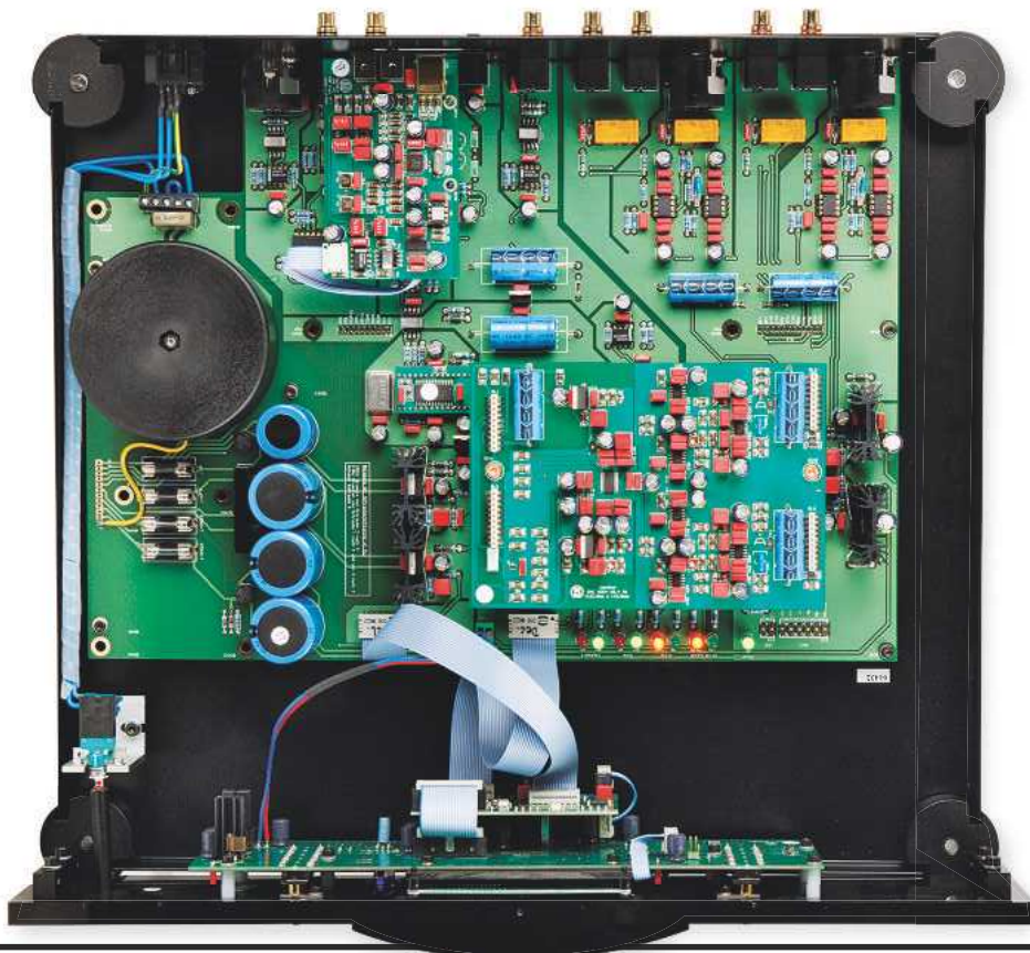
RIGHT: A work of art comprising full-sized and surface-mount components together with Crystal's popular CS4398 DAC. Note status LEDs for power, error, mute and de-emphasis
