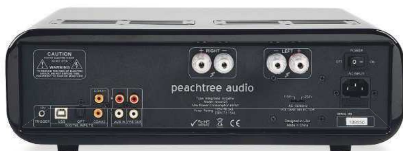
ABOVE: The Nova's 4mm speaker outlets are balanced (beware grounded speakers) with one analogue input, two digital coaxial, one optical and one asynchronous USB
