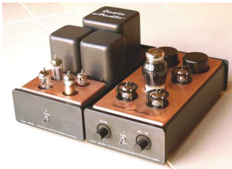
Early production photos. Showing PS3 upgraded version with JJ and Treasure valves, and Jensen Copper foil in paper and oil caps. Icon Audio MC transformers
