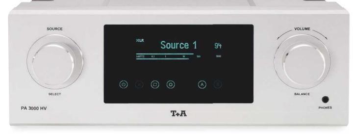
configured for bi-wiring or for driving a second pair of speakers. This is done via the amplifier's setup menu, where you can also name inputs, set trigger functions if required, and control the display brightness of the front panel VFD. A LAN socket is provided on the rear panel for computer control via automation systems.
