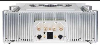
ABOVE: Unmarked, but explained in the manual, the right-hand RCA and XLR input(s) provide a non-inverting output, the left-hand RCA/XLR inputs an inverting output. Only one input may be used but the 4mm speaker outlets are paralleled for bi-wiring
