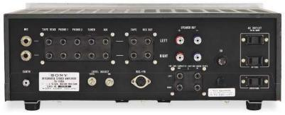
ABOVE: Only the two ¼in mic sockets differentiate the rear panel of the TA-1120A from many a modern amplifer. The pre/power amp links are absent in this picture
