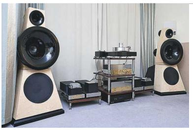
The Odeon No 38 horn speakers from Germany are not brand new, but they remain extremely popular with hi-fi show goers. Weighing 125kg each, they have a claimed sensitivity of 96dB and could be driven easily by the Jadis valve amps used here. A French Verdier turntable served as the only source for the system, giving the whole set-up real appeal to those who like to break with the norm. www. odeon-audio.com
