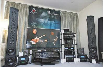
A real show-stopper was this multichannel system from McIntosh, the XRT1K speakers sporting no fewer than 28 tweeters. They were driven by MC2301 valve monoblocks said to be capable of delivering up to 300W into 8, 4 or 20hm. A real surprise came in the form of a new USB DAC/ digital preamp. Dubbed the D100, it fed hi-res tracks from a laptop to Sennheiser HD650 headphones [see p32]. www.mcintoshlabs.com
