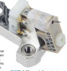
ABOVE: 3x70µm nude line contact stylus and solid boron rod cantilever. Colour-coded connections exit on flying leads while the body has three pre-tapped mounting holes
