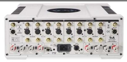
ABOVE: Note the dual-mono construction. There are six line inputs, four with balanced (XLR) options, plus a recorder in/out. Both balanced and single-ended (RCA) pre-outs are provided as well, along with two sets of speaker terminals for bi-wiring
