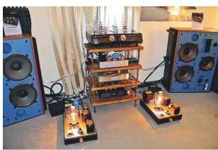
Russian tube amplification and acoustics specialist Next Sound came up with an unusual system. Vintage professional JBL 43 series speakers were driven by proprietary vacuum tube monoblock amplifiers and an active crossover. In terms of sound it was perhaps easily the best rock-oriented system of the show. www.next-sound.ru
