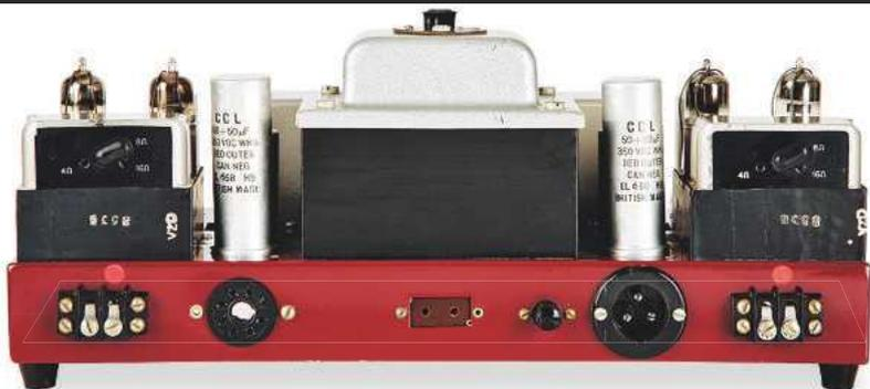
**ABOVE:** Rear view of the amplifier. The red dots that show loudspeaker phasing are a later addition, the original offering no clues. Beware the mains outlet (centre)
