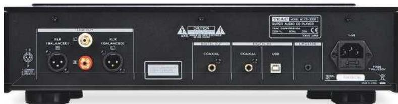
ABOVE: Balanced XLR output sockets are available in addition to RCA phonos. Two digital inputs are featured and one digital out. All of these feel extremely substantial
