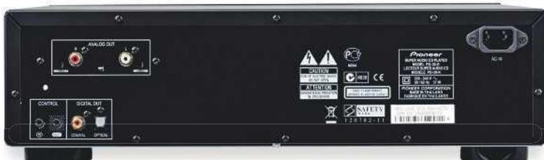
ABOVE: Single-ended (RCA) outputs for analogue and a pair of digital outputs (coax/optical) are grouped at one end, with the IEC mains socket at the other
