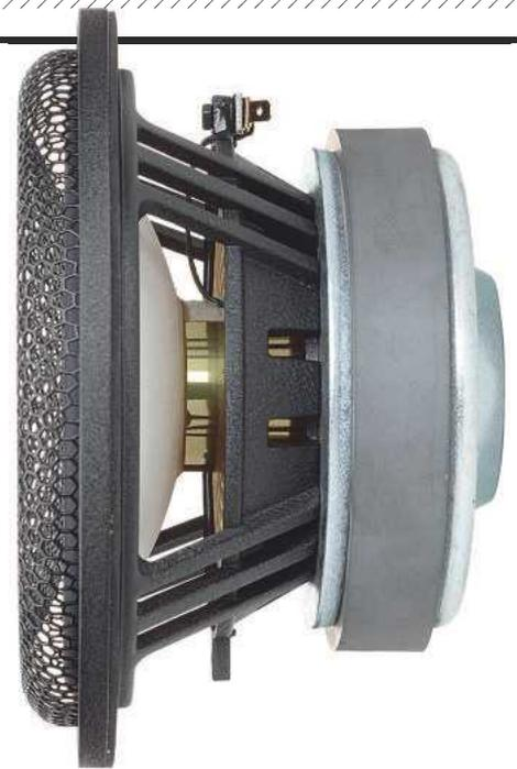
**ABOVE:** Side view of the 8in Accuton bass driver with its ultra-stiff ceramic/sandwich cone, thin fabric spider, underhung motor and 38mm titanium voice coil former
