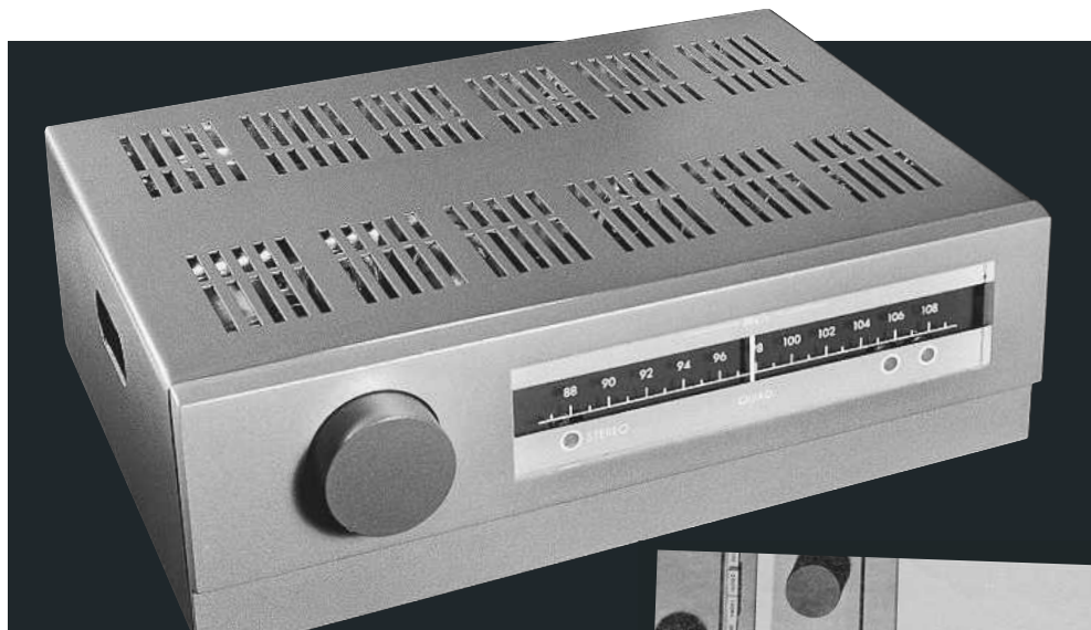
ABOVE: The Quad FM2 used a similar circuit to the original FM tuner. The later transistorised FM3 looks the same but lacks the vents in the top
