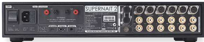
ABOVE: Phono sockets for five line level inputs, repeated via Naim's beloved DINs, plus an additional Aux 2 in and 4mm speaker outputs. There are also connections for a Naim external power supply, a USB port for firmware updates and remote socket
