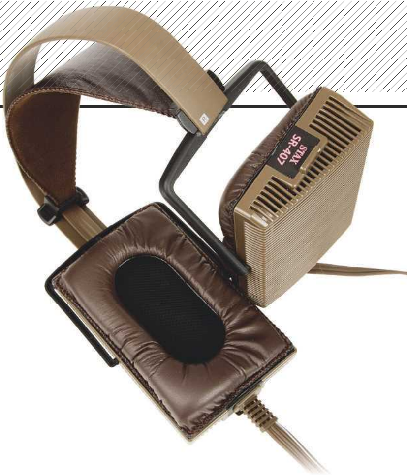
ABOVE: Flat cable carries DC polarising voltage for the diaphragms and the push-pull signals for the plates
