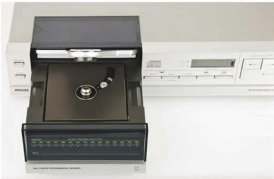
ABOVE: The Philips CD303, launched in the UK in late 1983. No flimsy plastic drawer here as the whole transport slides out on a sturdy assembly. Indicators on the front show the available tracks
