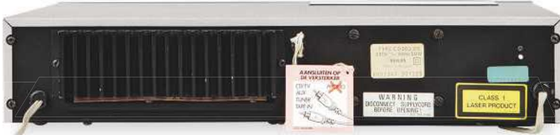
ABOVE: Rear view shows tethered cables and warning not to connect the player to the phono input of an amp, as owners replacing their LPs with CDs might have done
