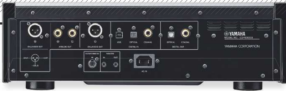
ABOVE: CD-S3000 has balanced XLR and single-ended RCA outs (both at 2V) with optical/coaxial S/PDIF and USB 2.0 digital inputs. BELOW: Inside, Yamaha employs a custom CD/SACD transport, separate digital/analogue PSUs, an ESS ES9018 DAC and fully balanced analogue output stages
