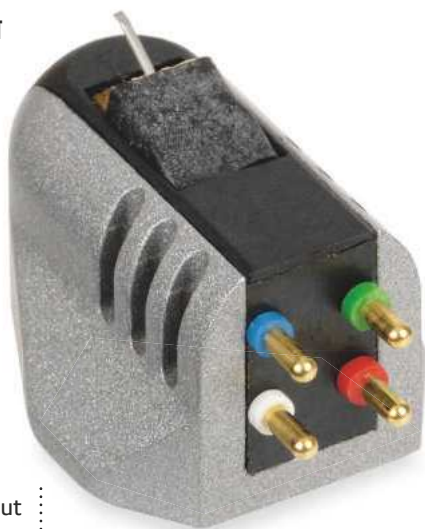
ABOVE: Hand-wound coils with a neodymium/iron/boron magnet meet an alloy cantilever and Vital stylus
