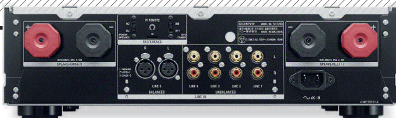
ABOVE: Massive 4mm speaker cable binding posts are joined by four single-ended (RCA) inputs and one balanced (XLR) input. This is a 'purist' line-only analogue amplifier with no USB or other digital inputs
