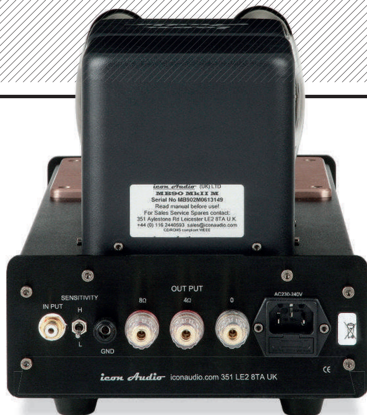
ABOVE: Rear socketry includes the usual 4 and 8ohm speaker connections, plus a switch to select High or Low sensitivity settings for the inputs. This helps make the amplifier suitable for use with passive preamplifiers too
