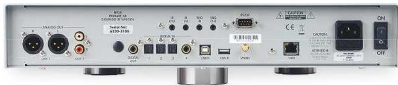
ABOVE: Four S/PDIF inputs and one output, asynchronous USB-B plus an iDevice-compatible USB-A input, trigger, external IR and RS232 – with XLR/RCA outputs
