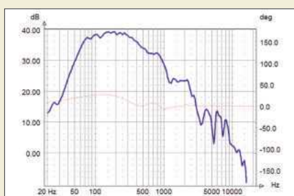
ABOVE: Near-field bass measurements of Sonus faber Venere 2.5 (top) and 3.0 (below)
