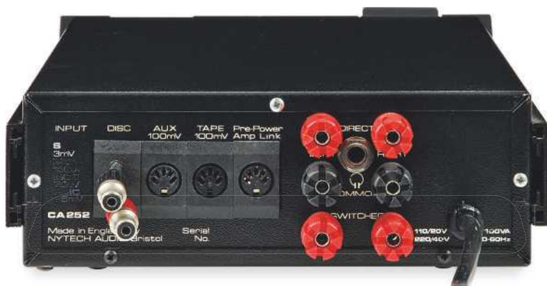
ABOVE: Rear view shows the flying leads for the turntable input and the almost inaccessible headphone socket. Other inputs are DIN, but work at close to line level
