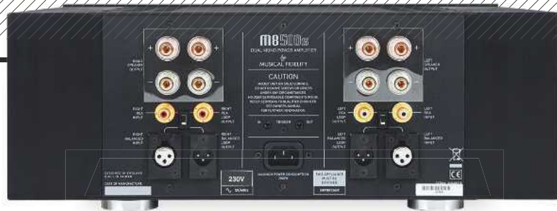
ABOVE: M8500s has two sets of speaker binding posts for bi-wiring and XLR and RCA loop-through sockets for easy bi-amping. 12V trig in/outs are also provided
