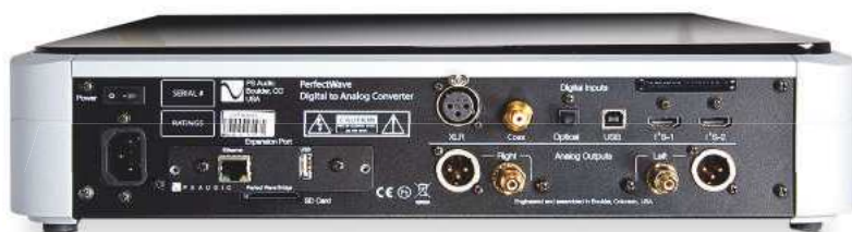
ABOVE: There are USB, coaxial and Toslink S/PDIF, and AES/EBU digital ins, plus I2S connections via HDMI, with RCA and XLR outs. Bridge module adds Ethernet
