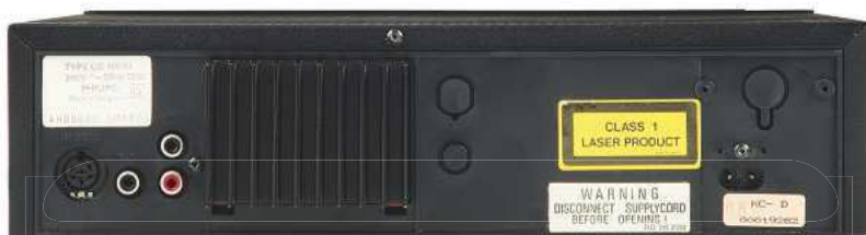
ABOVE: The rear panel, showing the analogue and S/PDIF outputs. The DIN socket is for a remote control receiver, though the player comes with one already built in
