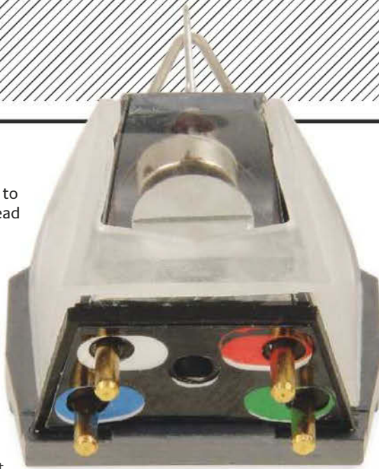
ABOVE: Seen through the Apheta's frosted acrylic wrap, the tiny moving-coil assembly with its lead-out wires is (just) visible in front of the magnet
