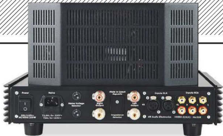
ABOVE: Four line-level inputs are offered, three unbalanced and one balanced. The cover between the speaker terminals hides loudspeaker impedance adjustments
