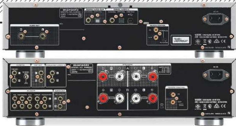
ABOVE: The player has USB, optical and coaxial digital ins, plus optical and coaxial digital outs; RCA line outs and remote bus sockets too. The amp has pre-out and power amp direct sockets, plus RCA inputs and binding posts for two pairs of speakers
