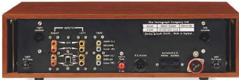
ABOVE: The rear view illustrates the usual problem of closely grouped RCA-type sockets into which some modern plugs will not fit. Note the cartridge loading switch
