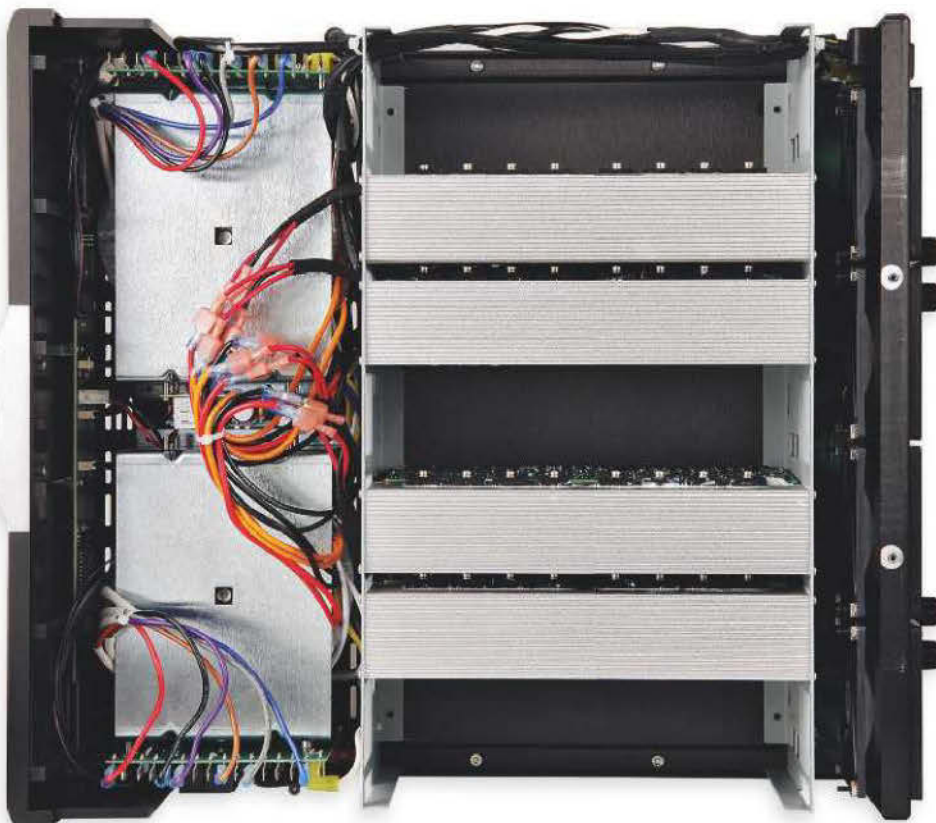
RIGHT: A dual-mono amp in a single chassis with two separately screened power supplies and no fewer than eight pairs of Motorola PowerBase 100W output transistors per side
