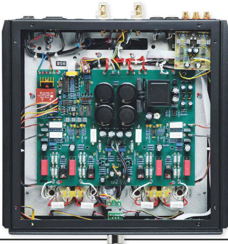
RIGHT: With the power and output coupling transformers encased in a steel box above, KR Audio's logic-controlled inputs, PSU smoothing, FET driver amp and volume are housed beneath
