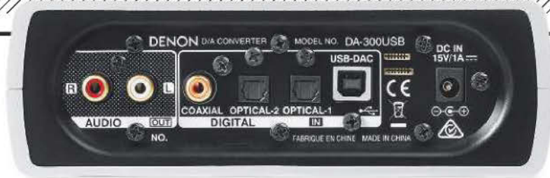
ABOVE: Self-evident sockets, so no need for the owner's manual: RCA phono line-out, one coax, one USB and two optical digital inputs, with DC power via a wall-wart
