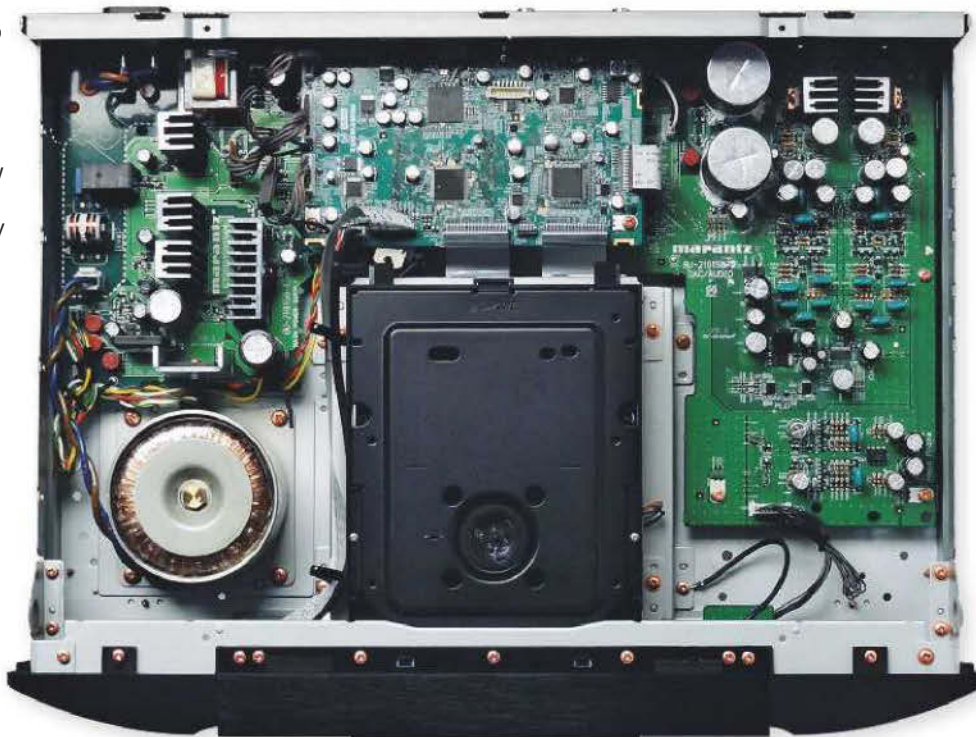
RIGHT: Three main PCBs (left to right) carry a switchmode PSU (for CD transport); S/PDIF and USB digital input reception; analogue PSU, DAC and preamp stage (black chassis version shown)
