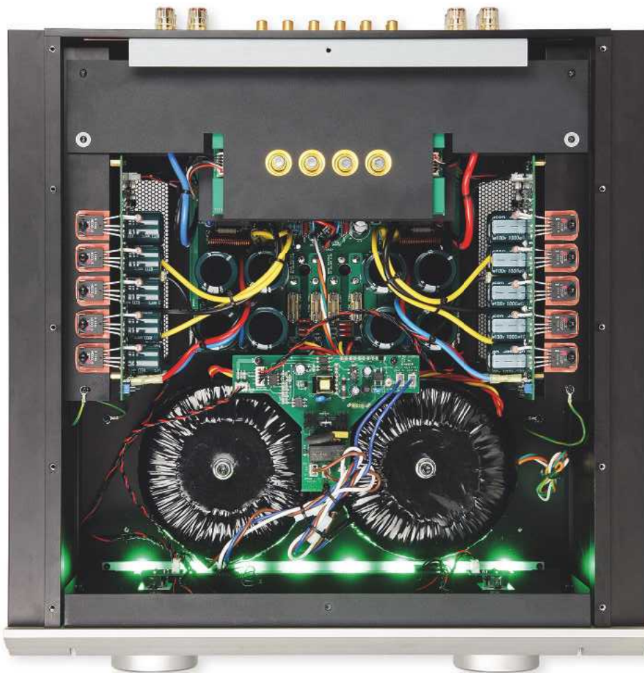
RIGHT: A pair of nuvistor triodes drive no fewer than five pairs of Sanken power transistors per channel. Note the pair of toroidal PSU transformers and dual-mono amplifier layout
