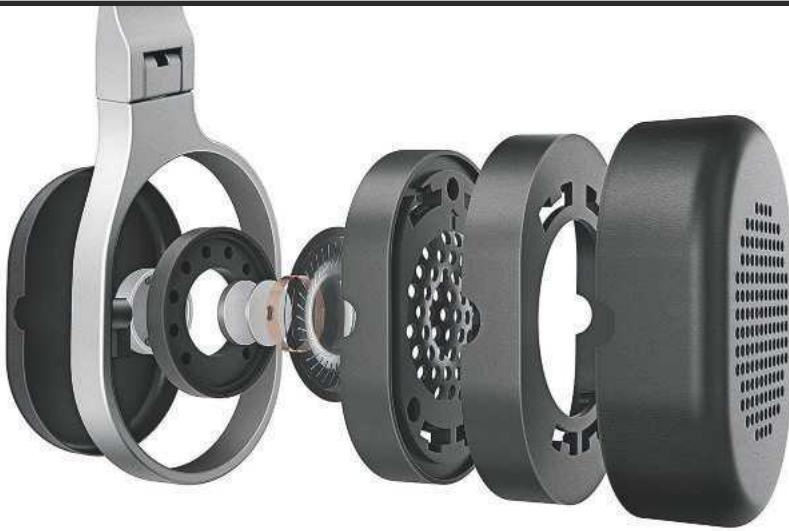
ABOVE: KEF's exploded diagram shows the aluminium alloy capsule frame, 40mm driver, acoustic tuning plate and supra-aural memory foam earpad
