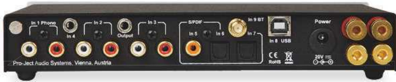
ABOVE: The back is crammed with three line, MM phono and five digital inputs, speaker terminals and a 3.5mm stereo line out, plus input for power from a wall wart
