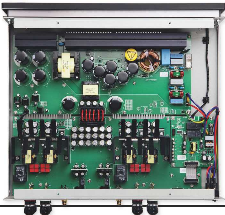
RIGHT: Primare's A60 power amplifier employs the most capable version yet of its proprietary UFPD Class D output stage, using two modules per channel in a balanced configuration
