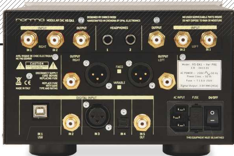
ABOVE: Rear panel layout reflects internal modular construction; digital inputs (USB, coaxial and Toslink S/PDIF, AES/EBU), and IEC mains at the bottom, DAC RCA and XLR analogue outs in the middle, and RCA analogue outs and headphone outputs above
