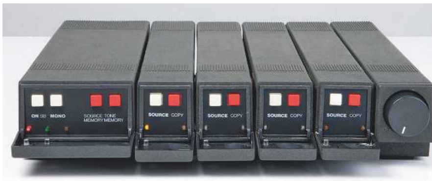
LEFT: Each module offered source and tape copy selection and could memorise switch-on source selection and tone control settings
