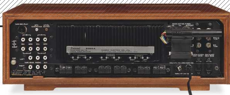
ABOVE: Well equipped rear panel is dominated by a large heatsink and connections for six loudspeakers. The damping switch is hidden behind the AM rod antenna
