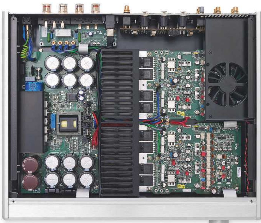
RIGHT: Exquisitely designed and laid out – with level-dependent forced air cooling – the PA 2000 R combines an efficient switchmode PSU with a derivation of T+A's 'High Voltage' amplification
