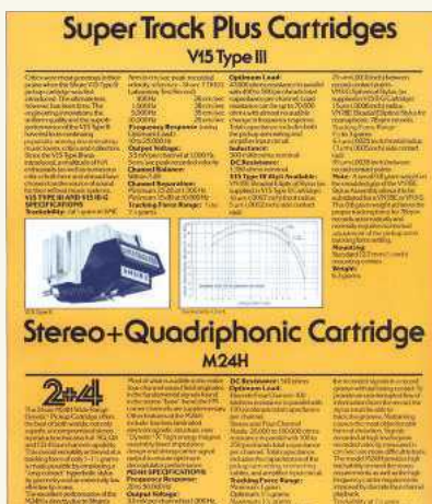
ABOVE: Shure suggests 400-500pF as the ideal load capacitance for its V15 Type III
