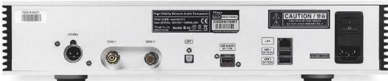
ABOVE: Aurender's N10 is equipped with AES/EBU, coaxial (RCA and BNC) and Toslink optical S/PDIF outputs, and one dedicated USB Audio Class 2.0 output. One Ethernet port and two USB 2.0 ports support network connectivity and file transfers
