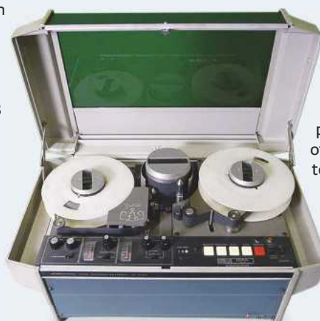
BELOW: IVC 800 videotape recorder from 1969 – a modified version was used by Decca's Bayliff and Griffiths
