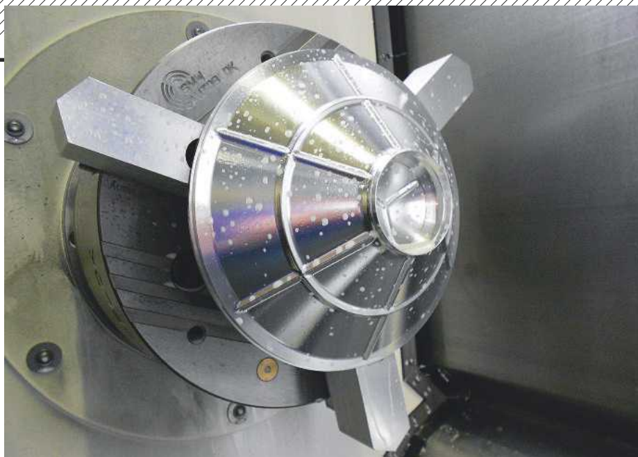
ABOVE: Every BilletCore woofer is machined in four stages that sees a 7kg cylindrical aluminium billet turned into a 35g cone. Here reinforcing ribs are retained on the rear of the BilletCore driver
