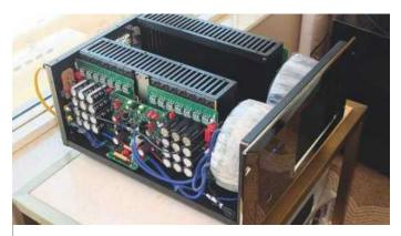
SAE is back with a beast of an amp! The 2HP is so-named because it's said to deliver 2x746W, or 'one horsepower per fully differential push/pull channel'. Another claim is that it is the quietest amplifier ever made, the engineers allegedly measuring it as having a >128dB signal-to-noise ratio. Our picture shows a prototype with polished steel fascia, but it's unlikely to reach production any time soon. www.hear-sae.com
