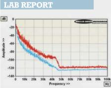
Offered here in its original 96kHz/24-bit recorded format, this BIS download shows full use of the available ~45kHz bandwidth and with good dynamic range too. There's only a hint of clipping with the loudest brass. PM
