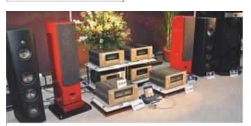
Two of Accuphase's new A-70 stereo power amps, seen at the front of this display, were set up to demonstrate Fostex G2000A and Magico Q3 loudspeakers. The A-70 is a Class A design, rated at 60W/ch and weighing in at 44.3kg. Also launched was the fully-loaded C-37 phono amp. *www.accuphase.co.jp*
