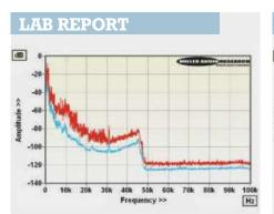
Cleanly recorded (aside from a signal at 31kHz) and with excellent dynamic range (the rise in ultrasonic noise is from the original – not an artefact of upsampling), this 96kHz file perfectly illustrates the 30kHz extension of a soprano voice. PM
