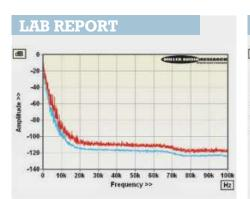
Sampling at 192kHz may seem excessive to record a piano with a harmonic bandwidth that rarely exceeds 20kHz, but the noise floor is exceptionally clean and the 'window' so wide it captures every ambient nuance. PM
