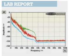
A genuine 96kHz recording but not without some 'hot' ultrasonic content [green trace, Graph above] that's as likely to be distortion from the percussion mic feed as true >20kHz harmonics. Some tracks also have a parasitic at ~38kHz. PM
