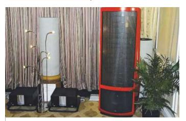
Powered by a pair of Krell Solo 375 amplifiers, the new MartinLogan Neolith hybrid electrostatics were delivering a suitably colossal sound. A combination of 15in and 12in woofers are married to a 48x22in mid/high frequency CLS XStat panel above 400Hz. www.martinlogan.com
