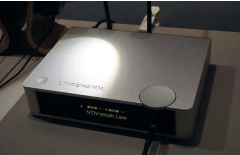
Lindemann's versatile Musicbook: DSD upsamples PCM files to higher resolutions or to DSD, while serving as a combination DAC, streamer, and preamplifier
