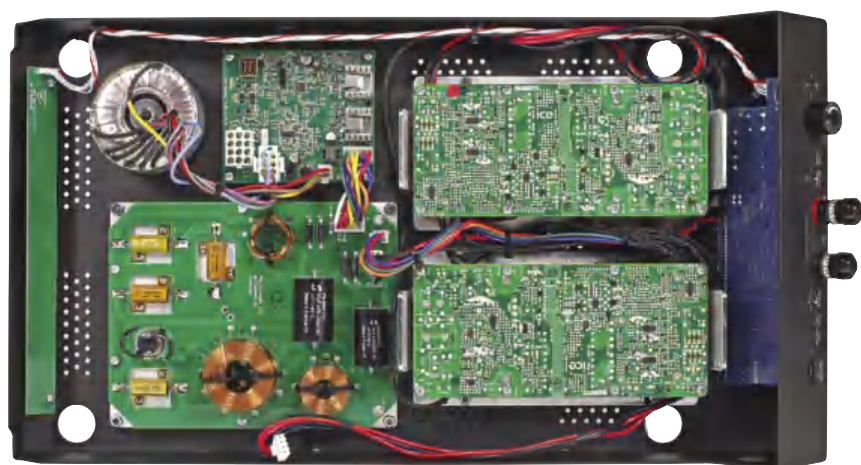
Inside the bottom tray lies a complex array of electronics, including two B&O Icepower Class D 500 Watt power amplifier boards (right), high and low voltage power supplies plus DSP (top) and an enormous crossover board with air core coils and polypropylene capacitors (bottom left).
