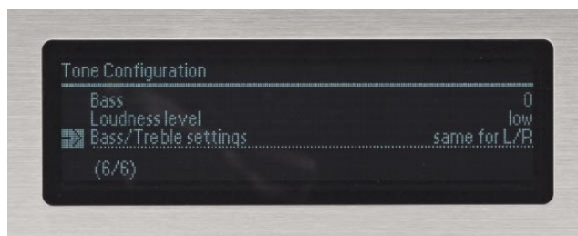
The bass/treble settings can be individually tailored for the left and right channels via the front panel.
