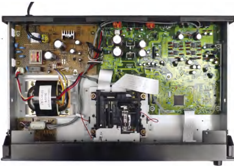
Most of the MDS-JB940 electronics is surface mounted. Service and instructional literature for the MDS-JB940 (and many other units) is freely-available from the excellent http://www.minidisc.org/ website
