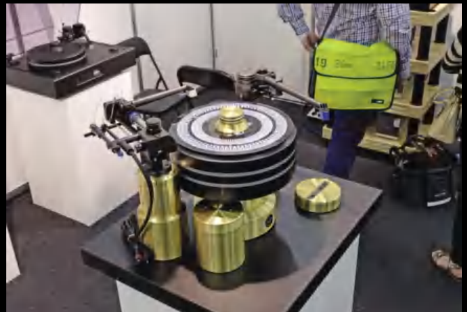
Kuzma of Slovenia ( www.kuzma.si ) are renowned for their exotic tonearms and turntables. They had a large stand at the show and on it was Air Line, a solidly built parallel tracking tonearm running on an air bearing. Parallel tracking eliminates geometric tracking distortion and the air bearing eliminates friction.
