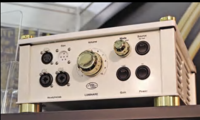
The Audio Valve Luminaire headphone amplifier: it even has an output for Stax electrostatic phones.
