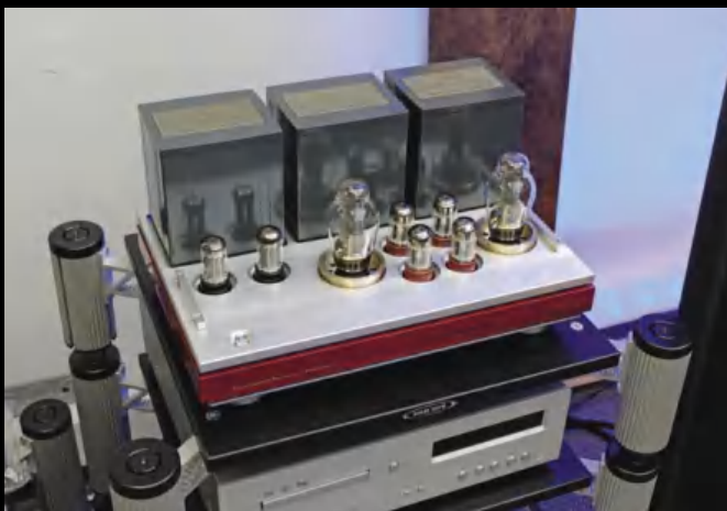
Luxman have returned to their roots, 31 years after producing their last valve amplifier, proudly announcing the MQ300 that uses 300B tubes in Single-Ended arrangement to produce a pure 8 Watts of Class A power per channel. Go to www.luxman.co.jp for this one and press the translate button.
