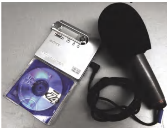
Here we have a typical 'off-the-shelf' bootlegging combo – a Sony MZ-N10 ('10th Anniversary Minidisc', circa 2003) and Sony ECM-MS907 'one-point' stereo microphone employing a 'mid-side' capsule configuration.
