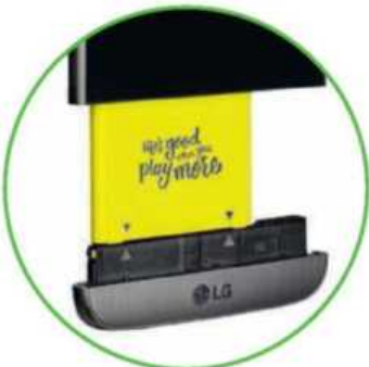
A detachable base allows you to swap the battery and add extra components
