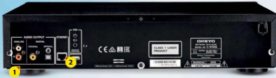
**1** When it comes to connecting to your amplifier, the Onkyo offers the standard choices of line-level for analogue and coaxial or optical for digital signals.
