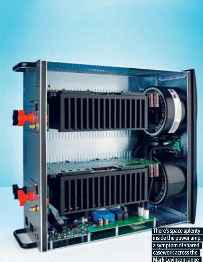
Dual transformers - one for the audio and one for the control circuits - help to minimise interference
