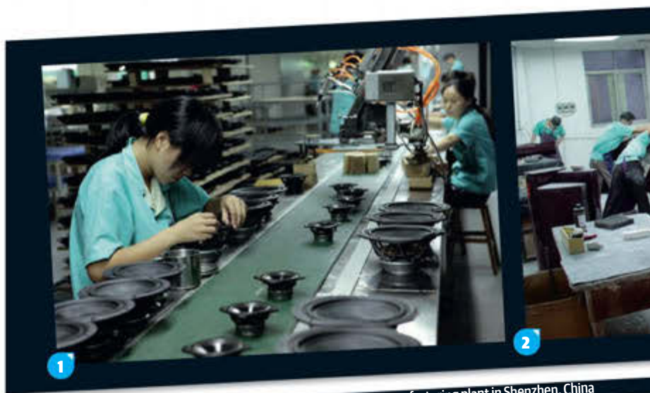
1 Driver assembly marks the start of speaker production at IAG's manufacturing plant in Shenzhen, China
