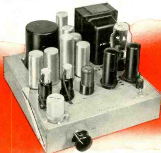
Monitoring Amplifier (Type BA-4A) —Designed for operation at microphone levels. High output of 12 watts is sufficient to drive several speakers or, in some applications, a recording head. Other uses include application as line amplifier for portable and mobile transmitters. High gain: 105 db. Low noise level: -20 db (with maximum gain); -40 db (with minimum gain). Low distortion: less than 3% at 12 watts. Frequency response: \pm 2 db, 30 to 15,000 cycles.
