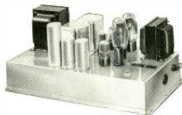
POWER AMPLIFIER CHASSIS — 16" x 10½" x 2" — base is steel, chromium plated and polished
