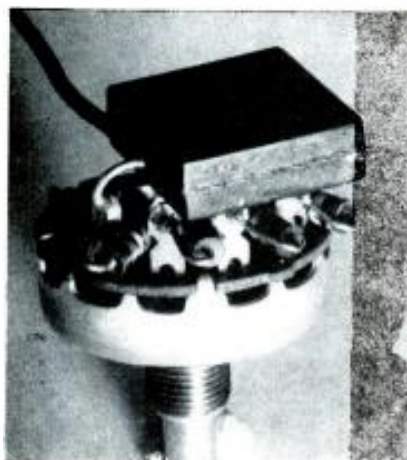
Fig. 4. Assembly of tone controls on standard switches to provide units easily wired into the control section. Left—bass control; right—treble control.
