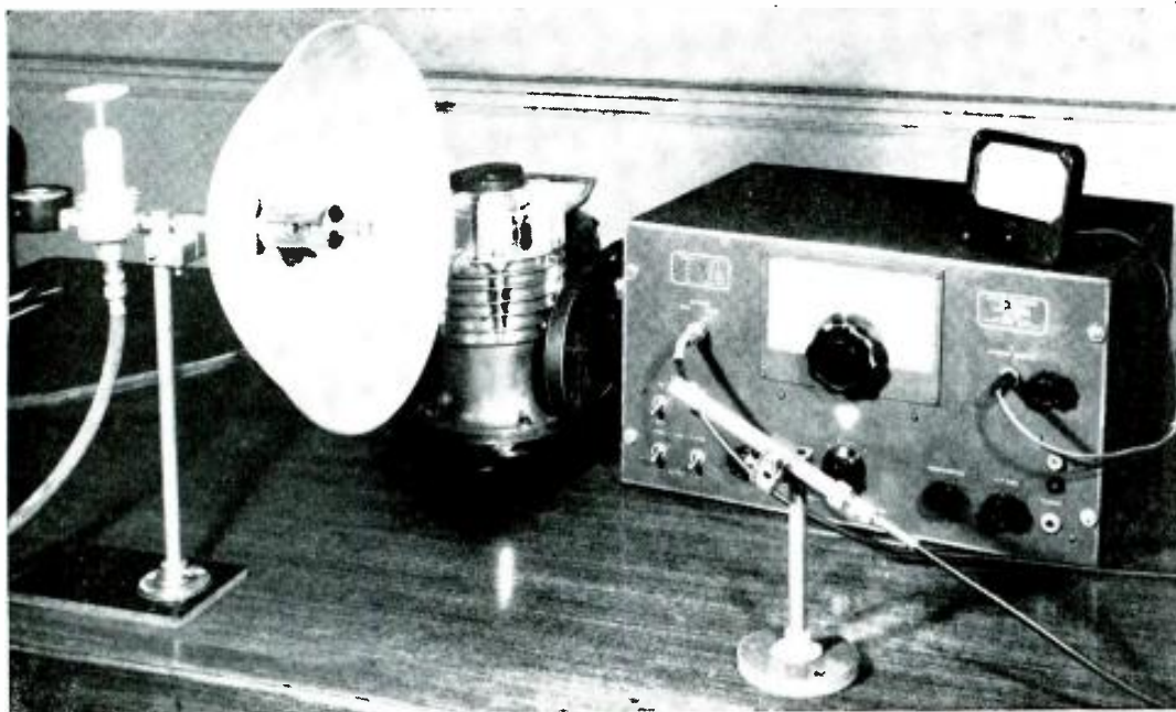
Testing Hartmann whistle in parabolic reflector.
