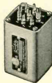
HIGH-FIDELITY INPUT TRANSFORMER, WF-20, for low impedance microphone, pickup or line to grid. Primary impedance 50, 125/150, 200, 250, 333, 500/600 ohms. Secondary impedance 50,000 ohms. Frequency response 30-20,000 cps. ± 2 db. Negligible harmonic and intermodulation distortion. Grey enamel cast case with phenolic terminal board and tapped holes for flush mounting. 2" high by 1¾" square.
