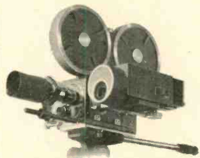
THE MAURER 16MM. , designed specifically for professional use, equipped with preci- sion high-power focusing and view-finder. Standard equipment includes: 235" dis- solving shutter, automatic fade control, view-finder, sunshade and filter holder, one 400-foot gear-driven film magazine, a 60-cycle 115-volt synchronous motor, one 8-frame handcrank, power cable and a lightweight carrying case.
