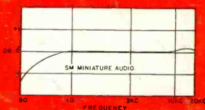
SM sub-miniature audio components, \frac{7}{16} " x \frac{1}{2} " x \frac{7}{16} " height. Weight — .009 lbs.
