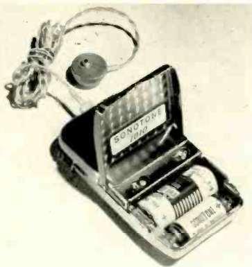
Fig. 3. Battery compartment provides space for both A- and B-batteries, and hinged door gives access to fitting controls.
