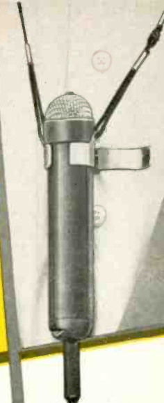
MODEL 646 DYNAMIC Small size. Response 40-14,000 cps, \pm 2.5 db in high range, specially compensated for chest operation. Power rating —57 db*. Omnidirectional. Integral blast filter. Choice of 50, 150 or 250 ohms. List, $140 Net, $84
