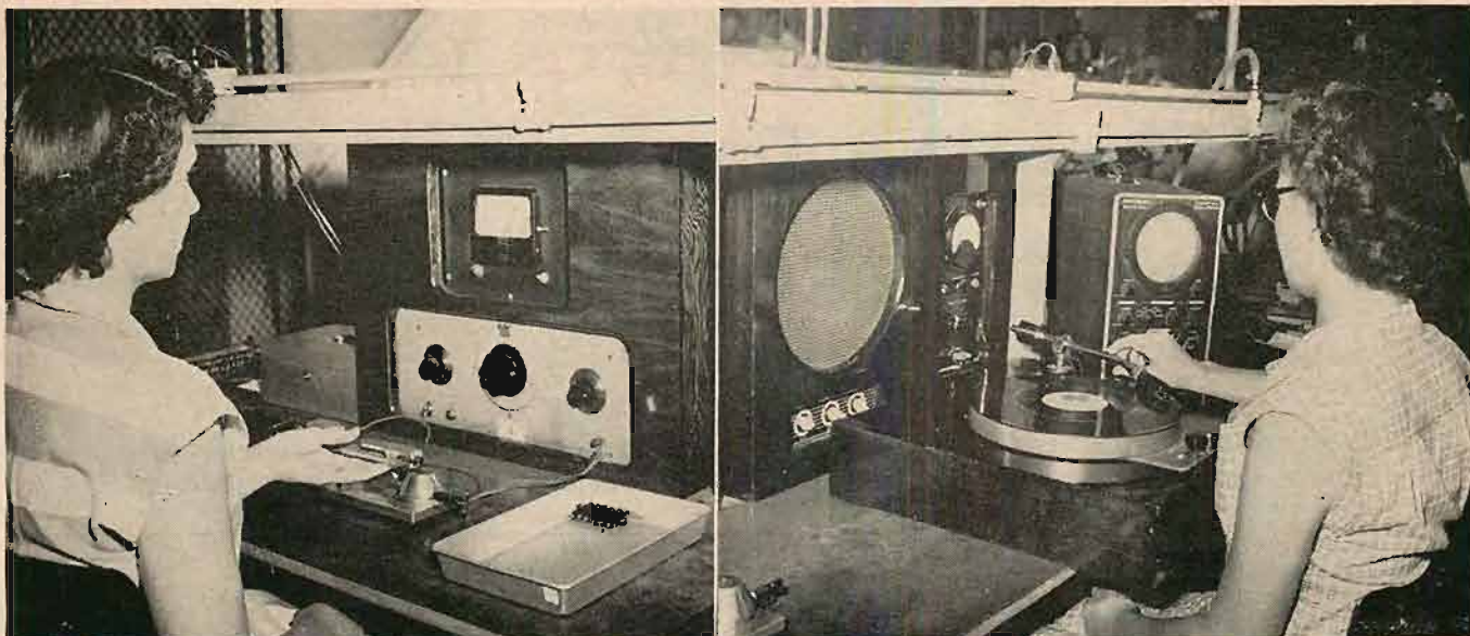
(Left) Production testing of compliance, using a magnetically driven vibrating reed which is loaded by the stiffness of the cartridge. The change in amplitude of vibration is read from the meter which is calibrated directly in compliance—the reciprocal of stiffness. A high value of compliance is necessary to prevent distortion and actual damage to the record groove. (Right) Production testing of output voltage and frequency response. Voltage output at 1000 cps is indicated on the meter while playing a test record, and frequency response is checked within a 2.5 db envelope on the face of the oscilloscope over the range from 50 to 10,000 cps. The source for this test is a sweep-frequency record.
