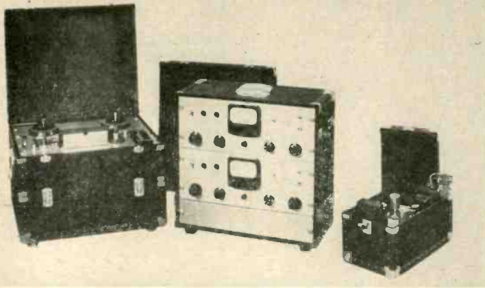
Fig. 4. A complete portable stereophonic recorder, with amplifiers and power supply.
