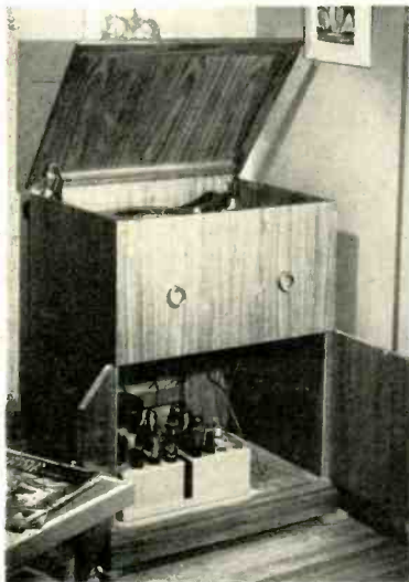
Typical cabinet housing the power amplifier in the lower portion, with a turntable and pickup and arm in the top along with the controls for the preamplifier which is custom-built and mounted directly on the motor board. (Courtesy Kierulff Sound Corp.)
